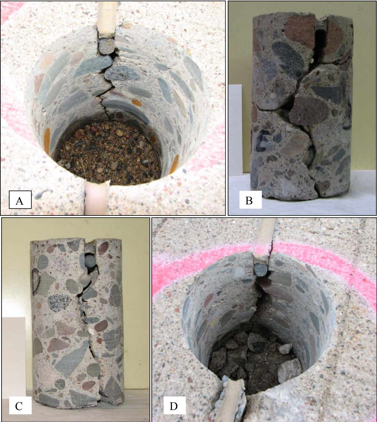
FIGURE 7 A) Core hole from cell 38, where joint sealant was in good condition; B) core hole from cell 38 where joint sealant was in poor condition; C) core from cell 40 where joint sealant was in good condition; D) core from cell 40 where joint sealant was in poor condition.
