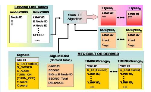
A travel time algorithm was implemented using the above schema to ultimately determine the travel time calculation using available signal information.
