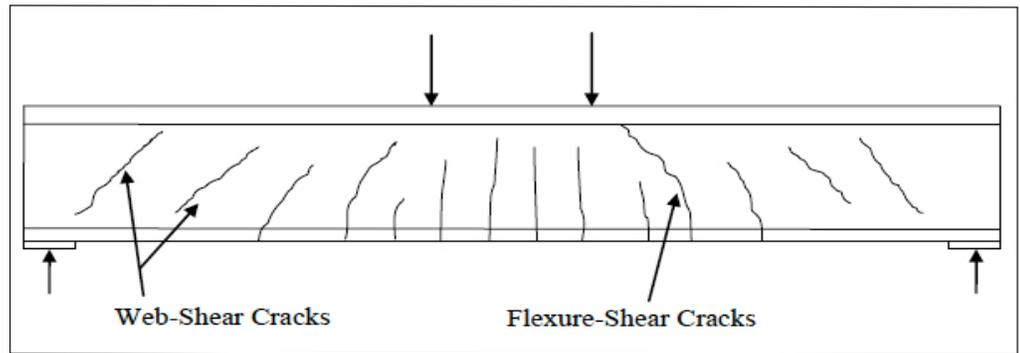
Excessive shear—the net force on a girder perpendicular to its length resulting from the pilings holding up the ends and the supported weight pushing down across the span—can crack the concrete of a girder, possibly compromising its strength.
