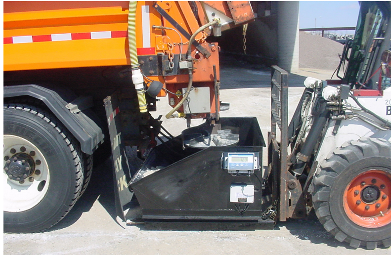
The weight box shown here is a simple-to-use tool that automatically weighs material for sander calibration. The weight box can collect approximately 500 pounds and requires a skid steer or forklift for positioning and emptying.
