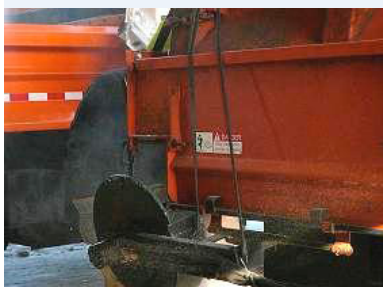
Tying up the spinner before filling the auger is part of the process to calibrate a manual sander controller.
