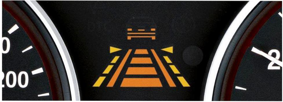
A vision-based lane departure warning system uses a camera and software to track and display a vehicle's position relative to lane markings, alerting the driver when a vehicle crosses markings at speeds greater than 25 mph or without a turn signal.
