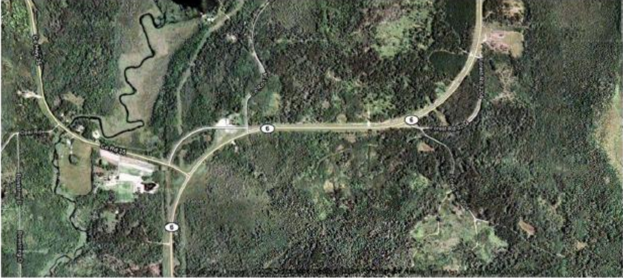
Figure 3.3 Aerial View of Flattened Curve on TH 6 (Source: Google Maps, ©2009 Google-Imagery ©Digital Globe, GeoEye, USDA Farm Service Agency, TerraMetrics Map data ©2009 Google). Both curves have been flattened; the former roadway is visible in both instances.
