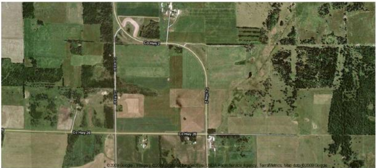
Figure 3.2 Aerial View of Flattened Curve on CSAH 2 (Source: Google Maps, ©2009 Google-Imagery ©Digital Globe, GeoEye, USDA Farm Service Agency, TerraMetrics Map data ©2009 Google). The 90 degree curve has been flattened; the former sharp curve is visible to the north east of the curve apex.
