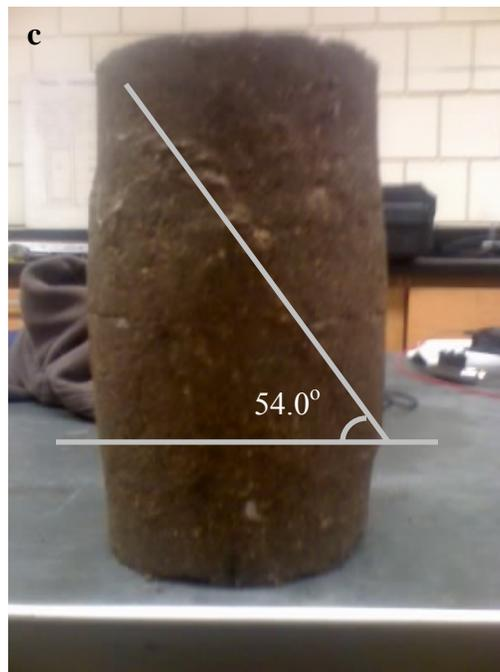
**Figure A35. Pictures of 50%RAP + 50%Aggregate mixture failed specimen during resilient modulus and shear strength testing for Fig. A35 a) and A35b) correspond to optimum moisture contents (<300 kPa suction), and Fig. A35c) correspond to water content at 300 kPa suction. Confining pressures were 1 psi for A35a and A35c specimens and 5psi for A 35b specimen.**
