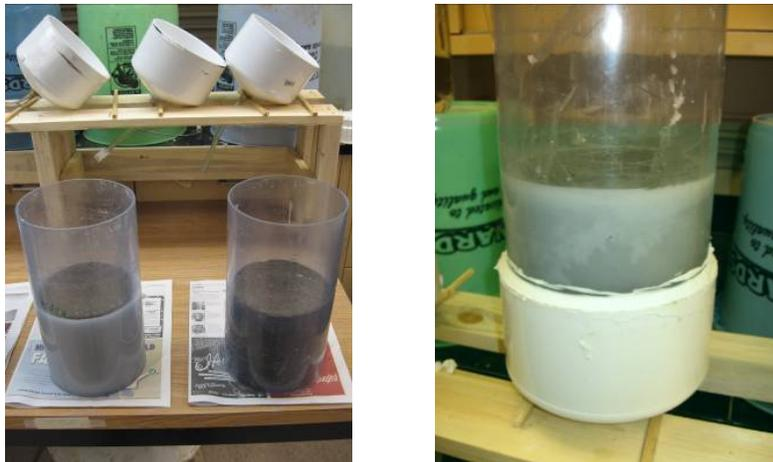
Figure 5.2 Assembly of specimens into leaching columns.
