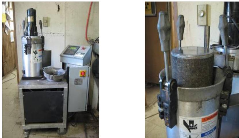
Figure 2.4 A gyratory compactor set-up.
