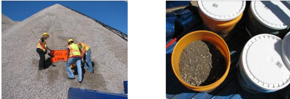
Figure 2.2 Recycled concrete material samples collected from a stockpile in the city of Minneapolis.
