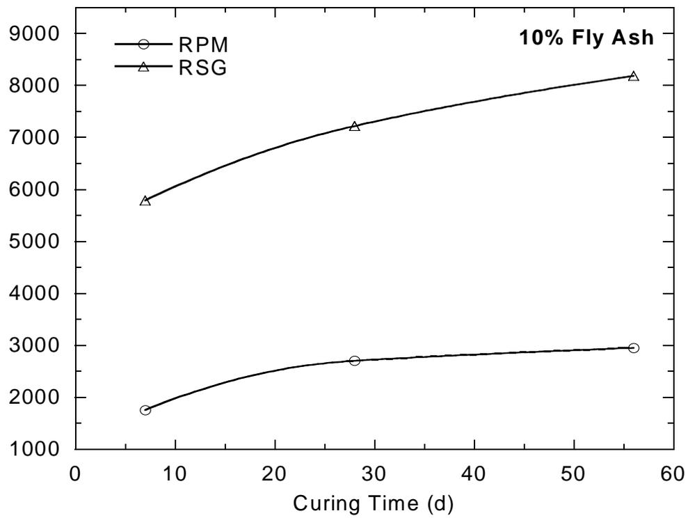
**Figure 8. Summary resilient modulus as function of curing time for SRPM and SRSG.**
