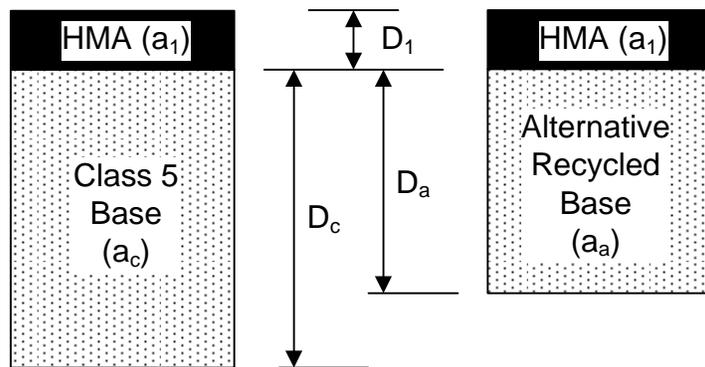
**Figure 3. Schematic of profiles for conventional pavement and alternative with recycled base material.**
