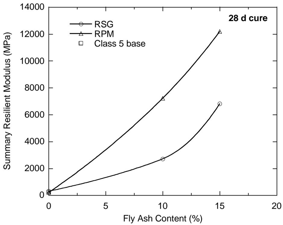
**Figure 6. Summary resilient modulus as function of fly ash content for SRPM and SRSG.**
