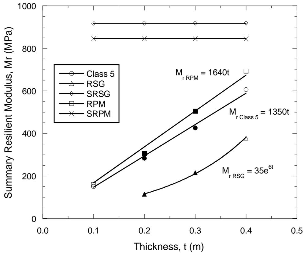
Figure 4. Summary resilient modulus of Class 5 base, RPM, RSG, SRPM, and SRSG as a function of base course thickness.
