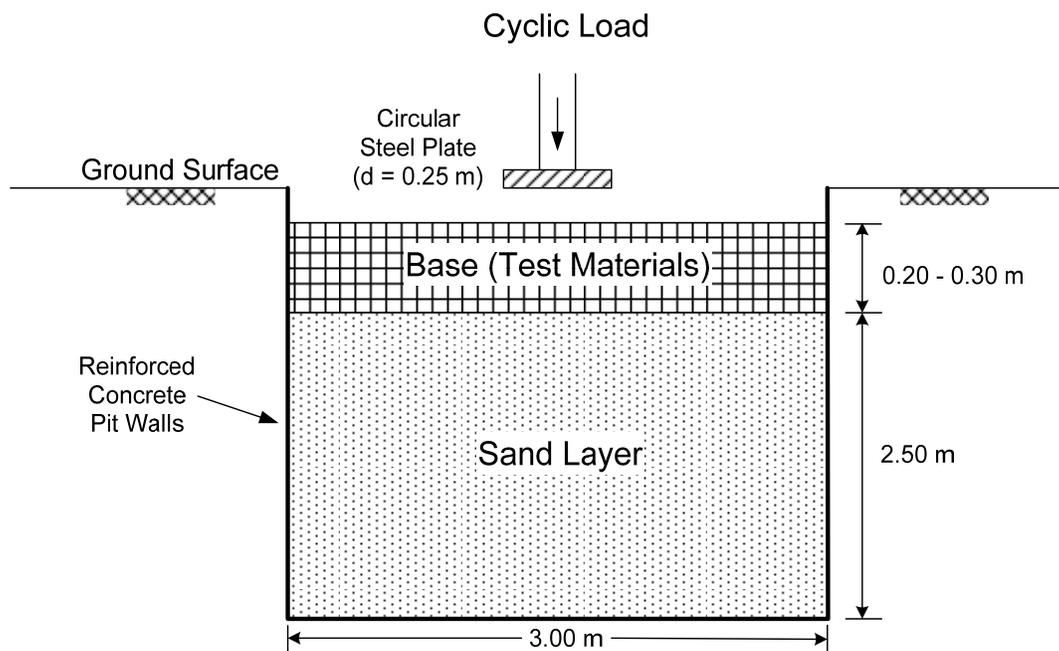
**Figure 2. Schematic of LSME used for prototype testing and evaluation.**
