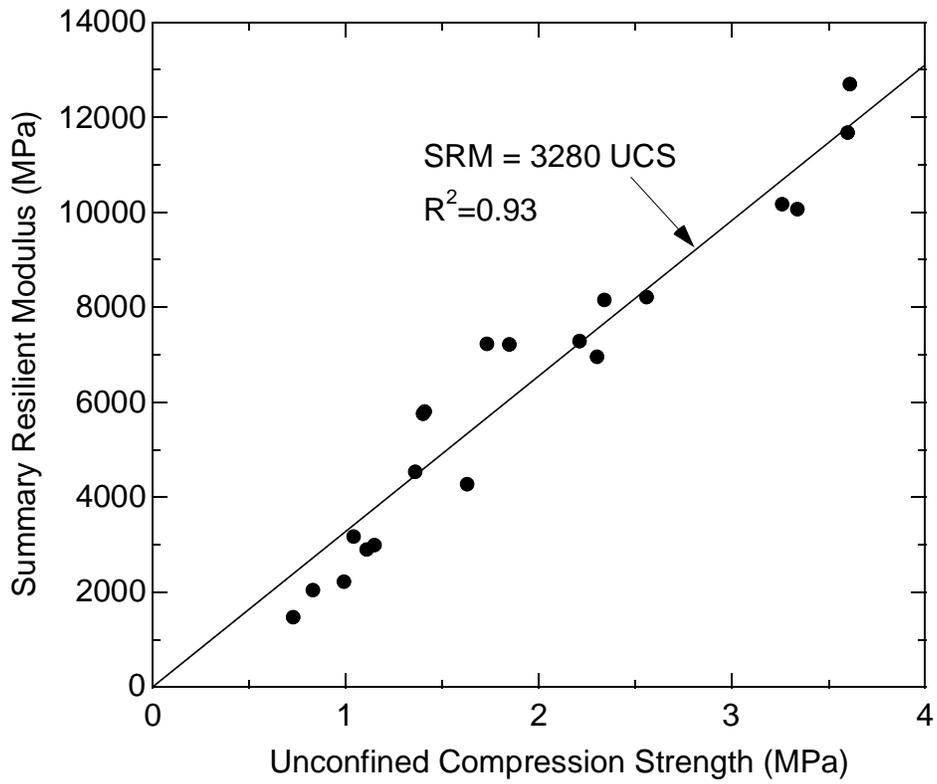
**Figure 7. Summary resilient modulus of SRPM and SRSG as a function of unconfined compressive strength.**
