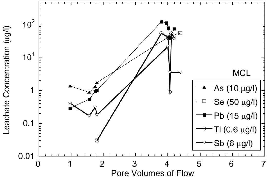
Figure 9. Concentrations of select trace elements in lysimeter at Waseca site.
