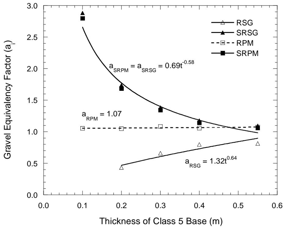
Figure 5. Gravel equivalency factor for RPM, RSG, SRPM, and SRSG as a function of thickness of Class 5 base.
