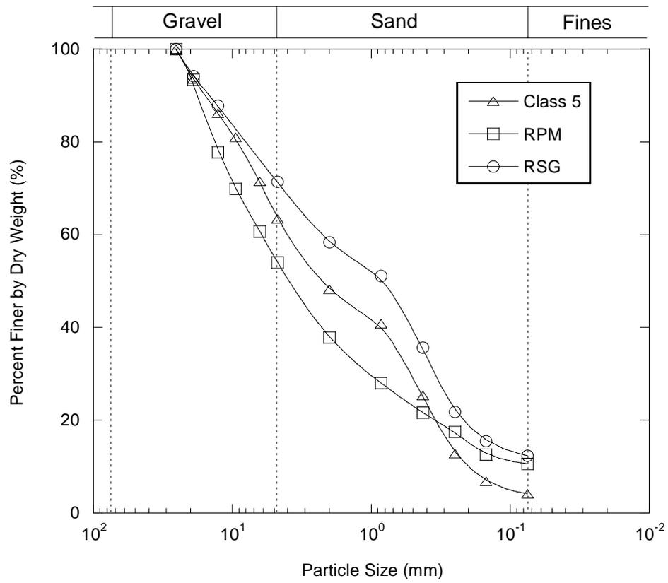
**Figure 1. Particle size distributions of Class 5 base, RPM, and RSG used in study.**
