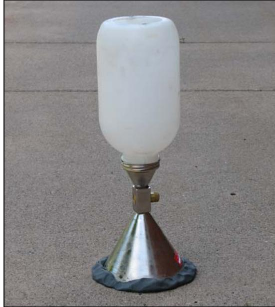
**FIGURE 7: In-situ drainability measurement device.**
