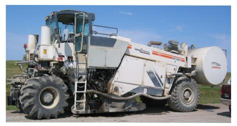
Foamed asphalt machines such as this one are used to pulverize the road surface and inject it with a foamed asphalt mixture that can be compacted on the roadway to form a new surface.
