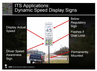
The workshop provides guidance on safety tools such as dynamic speed display signs. A presented study showed that drivers on average slowed by approximately 7 mph after these signs were installed at five sites.
