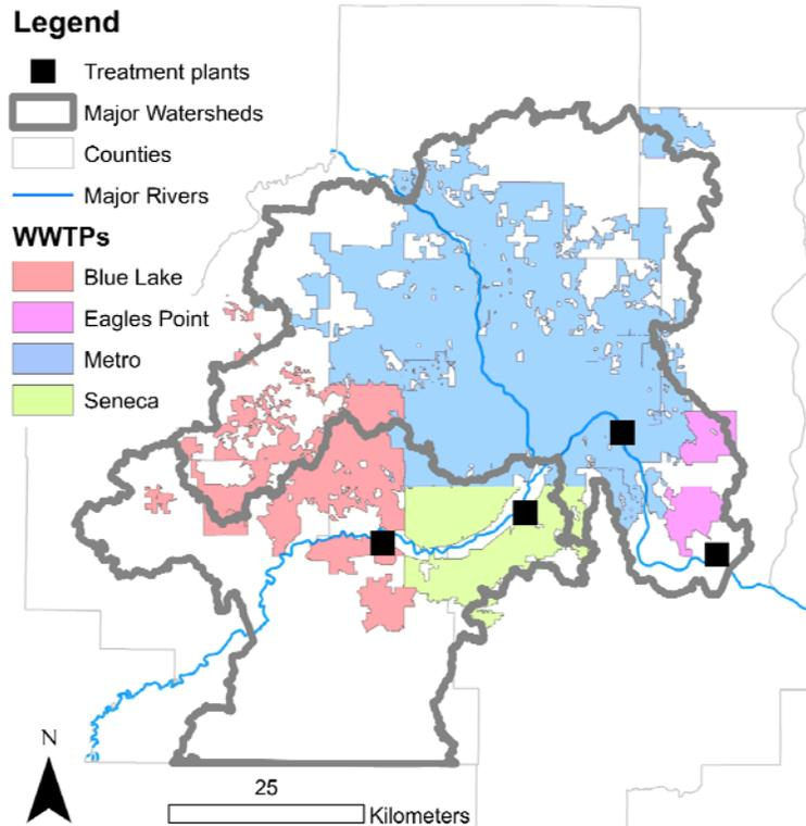
**Figure 3.6 Coverage of the four WWTPs discharging into the watershed. Data layers obtained from Metropolitan Council GIS database.**
