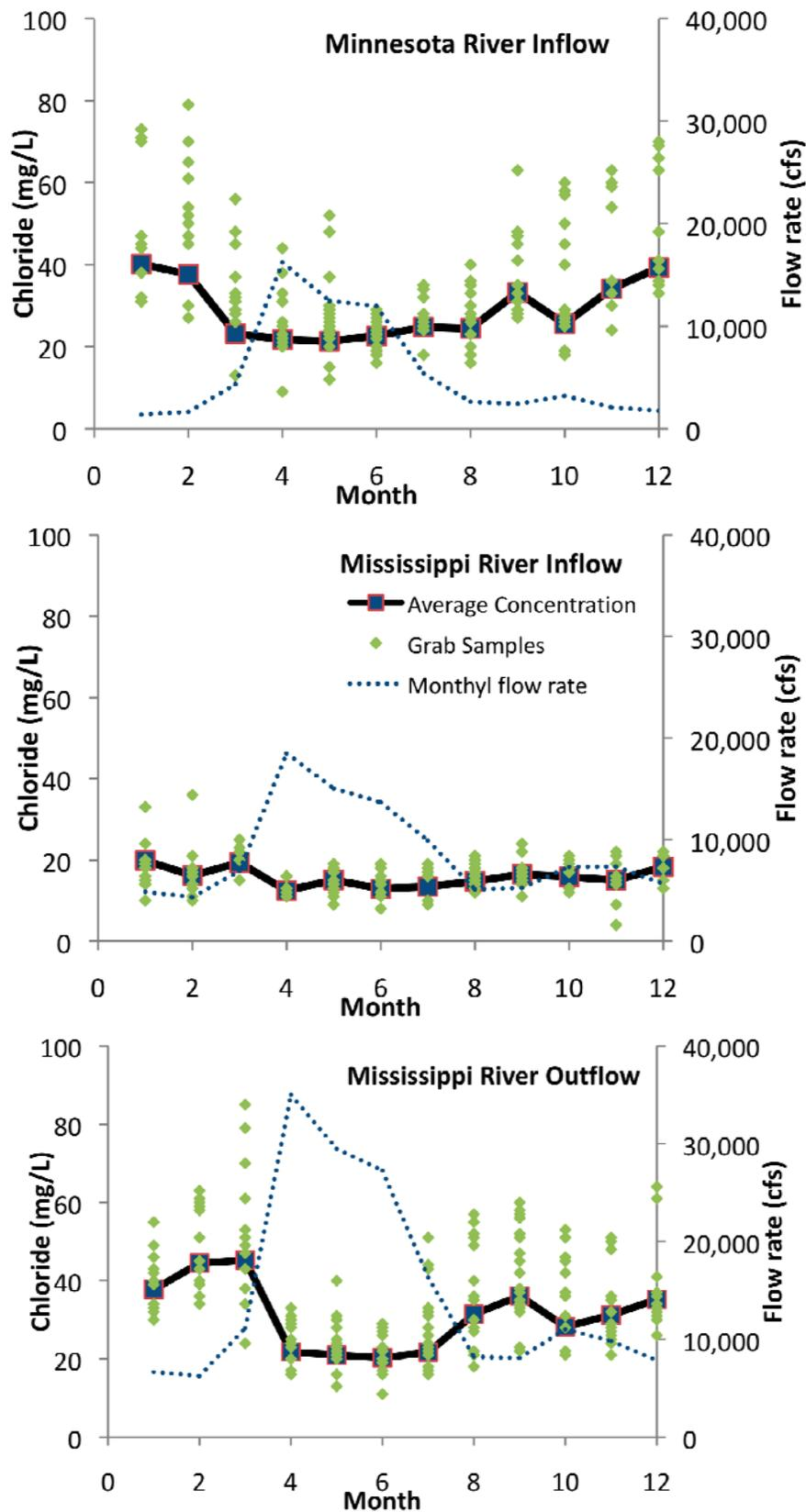
**Figure 3.3 Chloride concentrations in individual grab samples from the Minnesota and Mississippi Rivers. Flow-weighted average monthly values for concentrations and flow rates are plotted as solid and dotted lines, respectively. All values are from measurements taken between the years 2000 and 2007.**
