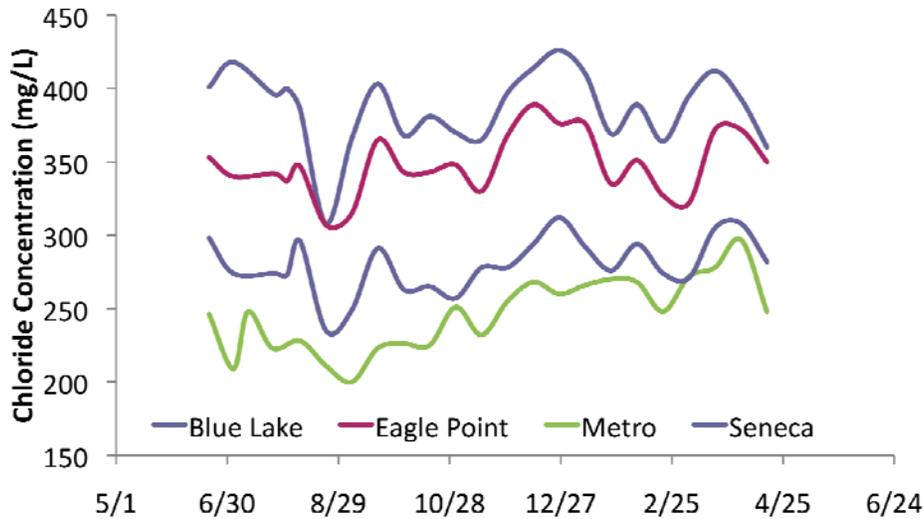
**Figure 3.7 Chloride concentrations in WWTP effluents (June 2007-May 2008).**
