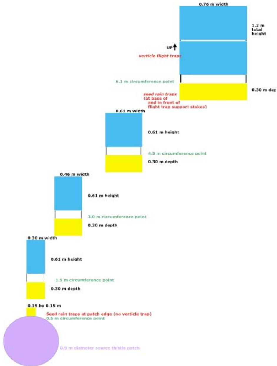
Figure 2. Spiral trap dimensions and layout. One spiral is shown.
