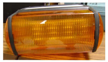
Compared to the standard HID strobe light, LED emergency strobes (above) are not as visible from as many different angles of driver approach, possibly creating safety issues.
