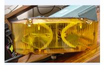
The standard emergency lighting currently used on Mn/DOT snow-plows consists of an HID strobe light like the one shown here.
