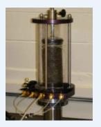
Researchers compared the stiffness of unbound and stabilized material samples by testing resilient modulus confining pressures in triaxial cells.
