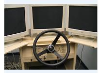
The STISIM simulator uses three PCs to generate a virtual environment presented on 17-inch monitors.
