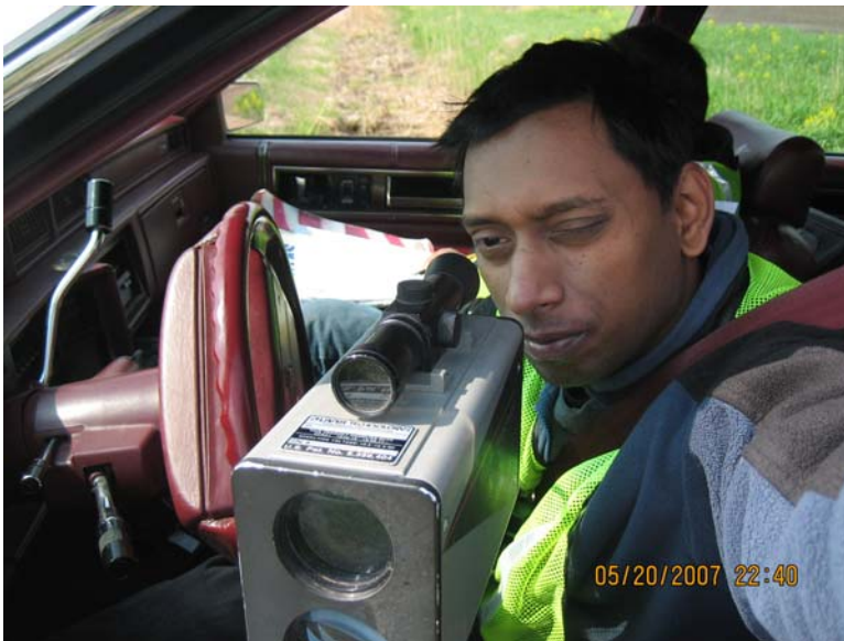
Figure 4.31. Use of a laser gun to collect spot speeds.
