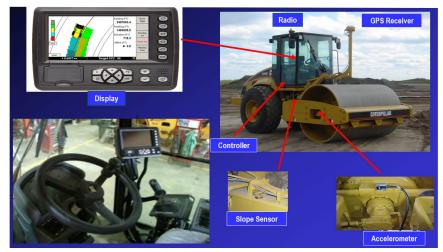
IC rollers include accelerometers mounted on their drums to monitor vibration amplitudes and frequencies. An on-board electronic display system exhibits a colorcoded map of stiffness data analyzed in real time to identify weak areas under the soil.
