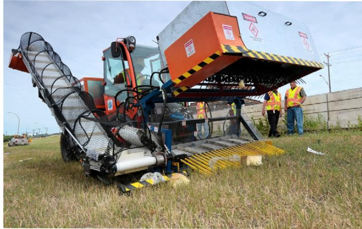
The trash-harvester prototype developed for this study has a Holden tractor for its core. The front pickup unit lowers onto the tines to scoop up litter and sweep it to a conveyor belt on the right side.
