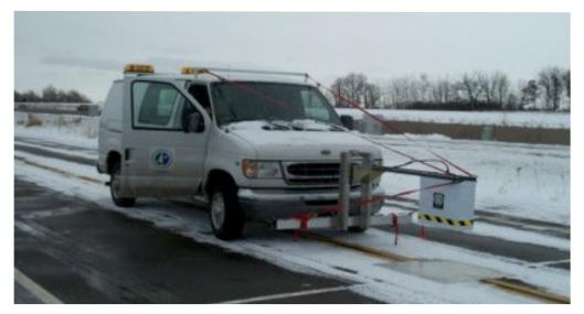
GPR is mounted on a van and gathers pavement structural data, such as thickness, at 50 mph so workers don't need to close traffic lanes to cut out multiple pavement samples.
