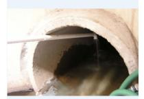
Researchers fed sand and water from fire hydrants into stormwater systems to see how underground drainage systems distribute suspended solids.
