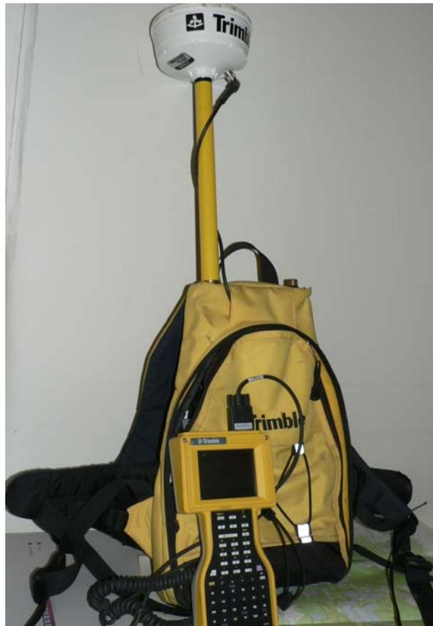
**Figure E1:** *Trimble® PRO XR GPS Unit used in the survey and data recording phases of the study.*
