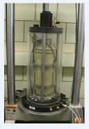
Laboratory stiffness testing involves recording the response of a sample of base material in a pressure vessel to a series of loads.
