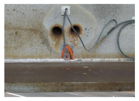
Figure 7-29: Photograph of Web Gap Strain Gage Vertically Aligned on Web
