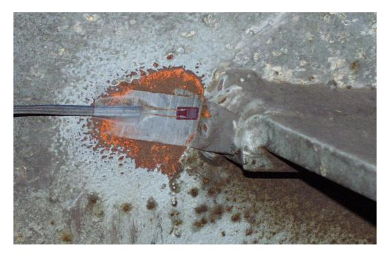
Figure 7-25: Photograph of Gusset Plate Tip Strain Gage
