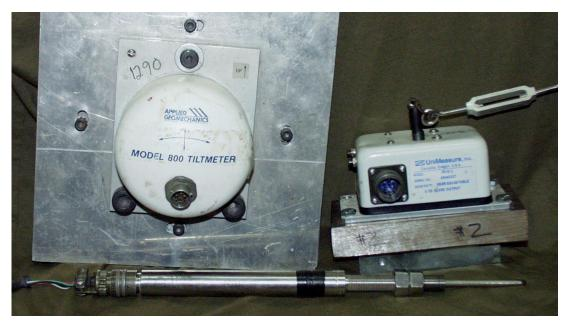
Figure 5-3: Tiltmeter, String Potentiometer, and LVDT used for Test Displacement Measurements
