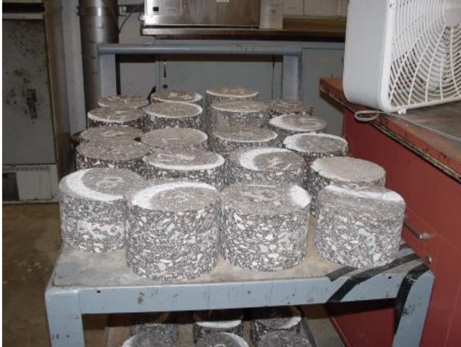
**Figure 1.8. MnROAD Cores of Variable Thickness**
