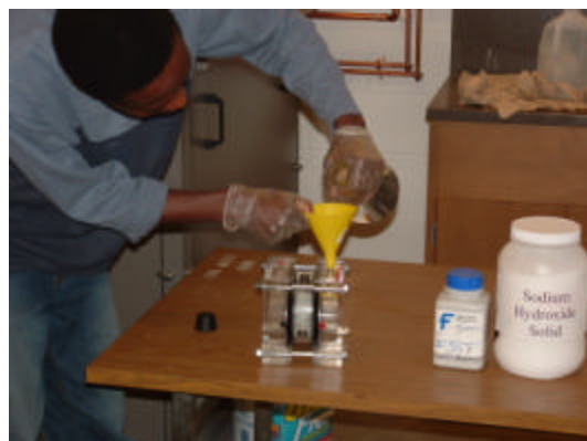
(b) Filling cell reservoirs
