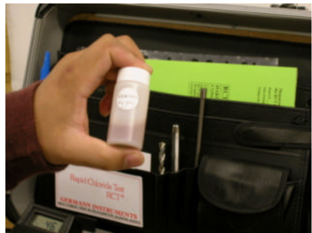
Figure 3.5: Rapid chloride test setup
