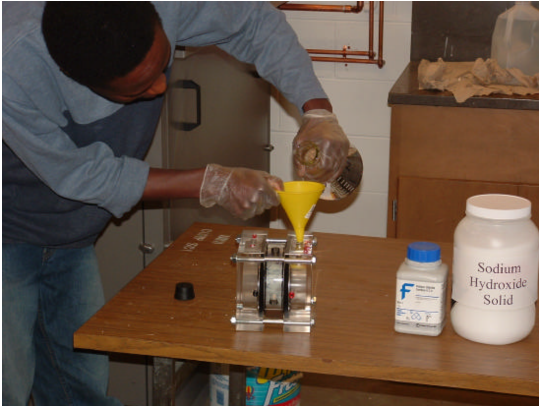
Figure 2.2: Concrete specimen mounted inside the RCPT cell.
