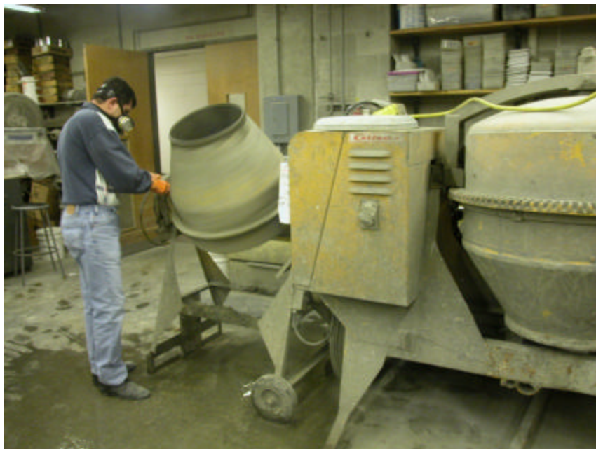
Figure 4.2: The 5-ft 3 concrete mixer used to prepare fresh concrete
