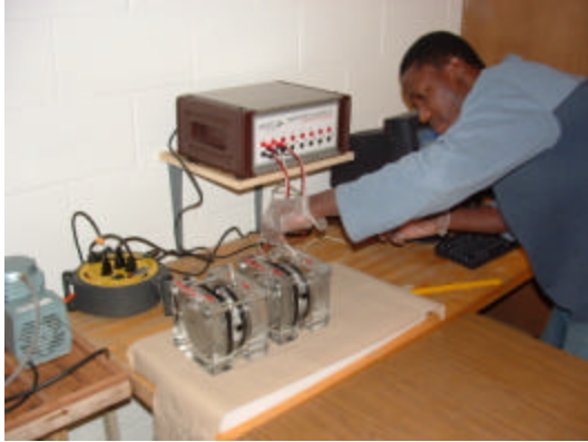
(c) Connecting cell to data acquisition system
