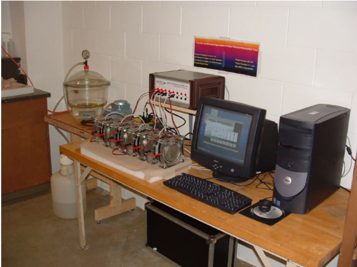
Figure 2.1: Rapid chloride permeability test setup at UWM
