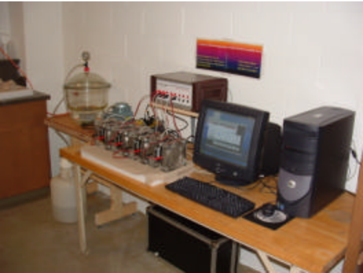
(e) Running RCPT on 4 concrete specimens
