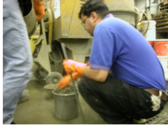
(b) Compacting concrete in the bowl
