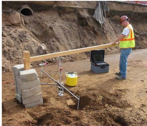
Plate Load Test Equipment
