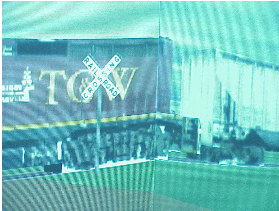
Figure 2-4. Simulated train crossing HRI with passive Xing crossbuck sign
