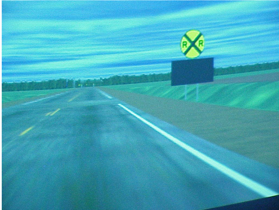
Figure 2-8. Simulated active advance VMS
