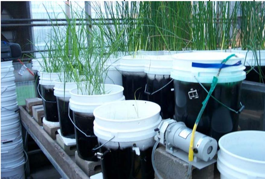
In Figure 3.2, please note that the reactors are set at slightly different heights from each other. Each reactor is connected to its two neighbors at their respective water lines. So, any excess water in the first reactor flows into the second reactor, and so on. The nutrient solution drains at the set flow rate from the bottom of the reactor and a series of tubes is connected to the
