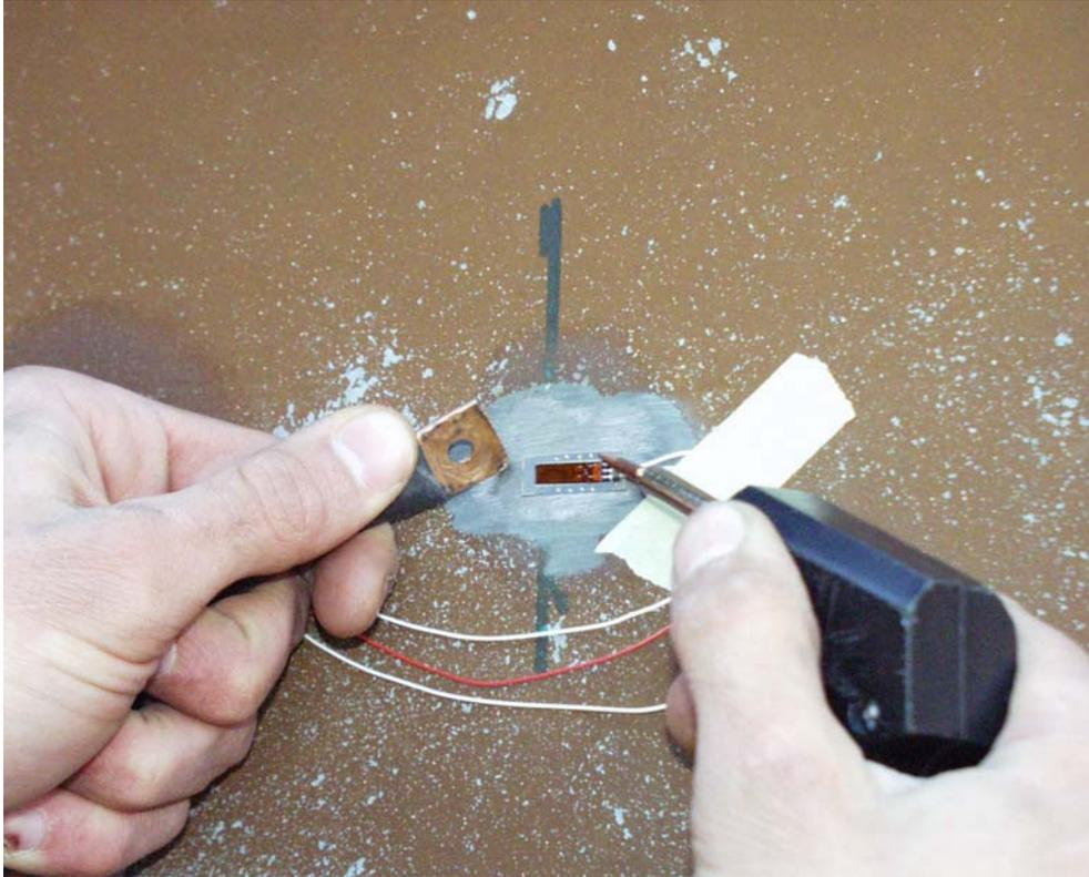
**Figure 3.1: Welding of a strain gage**
