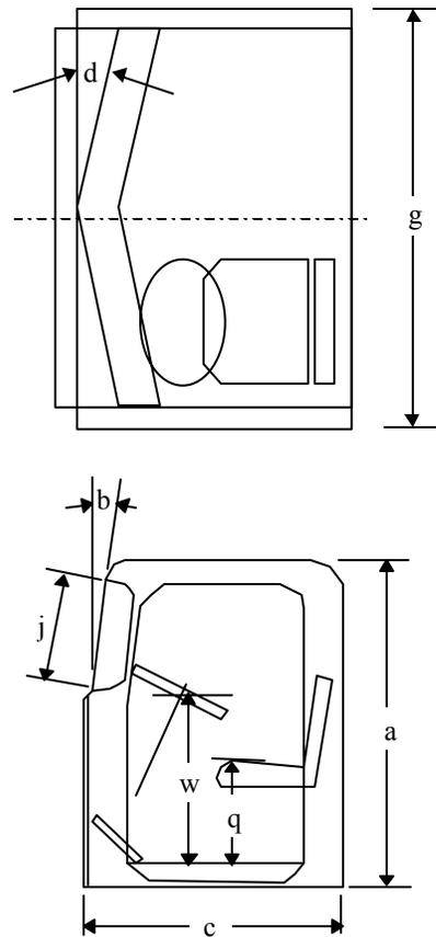
**Figure 17. Dimensions of the truck cab.**
