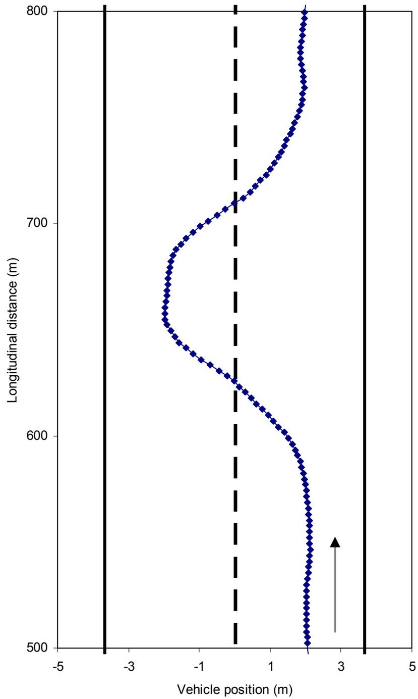
**Figure 54. Vehicle position along with the driving lane. Note: the scale factor for the vehicle lateral position axis, i.e. X-axis, is greater than the scale factor for the vehicle distance along the longitudinal direction, i.e. Y-axis.**
