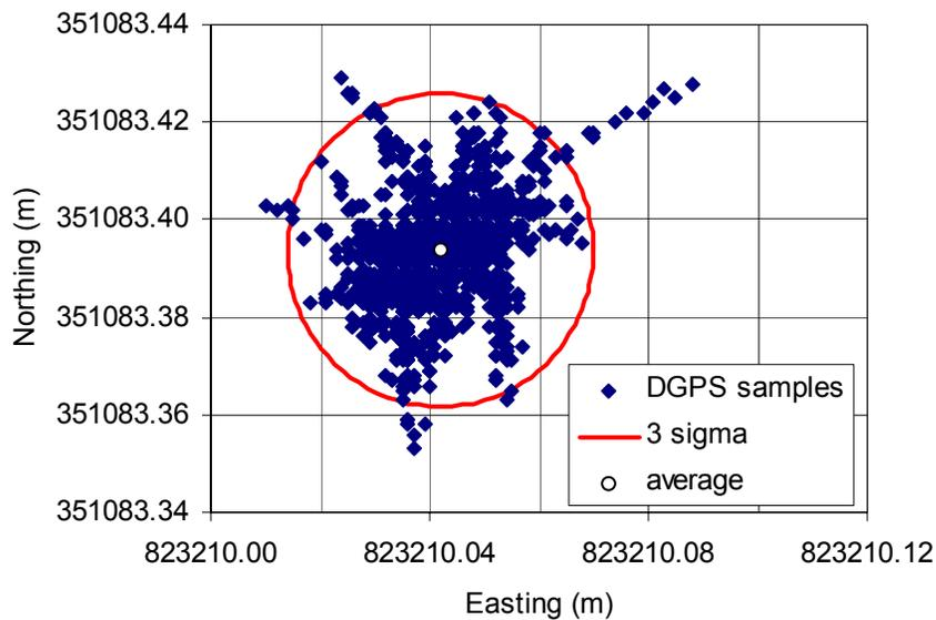
**Figure 48. Sample data from a stationary DGPS receiver (Novatel RT20).**
