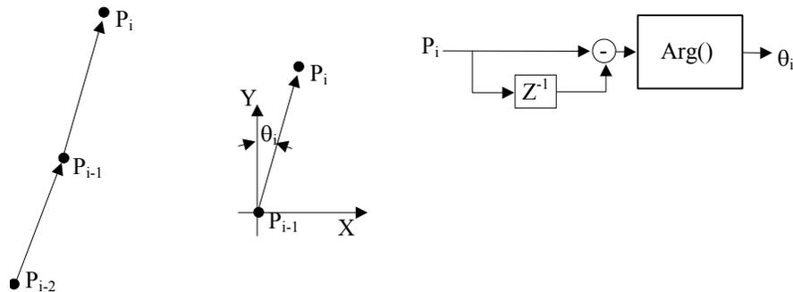
**Figure 47. Yaw angle estimation for linear motion.**
