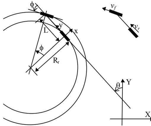
**Figure 42. The bicycle kinematics model.**
