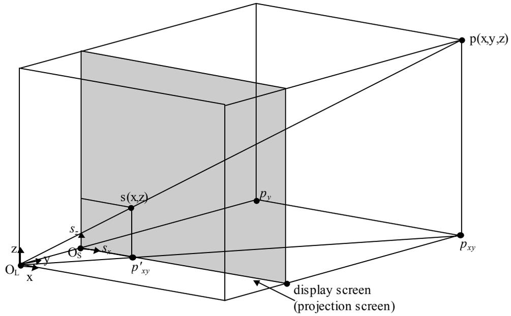
**Figure 32. Geometry of perspective projection.**
