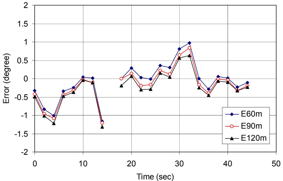
**Figure 62. Effect on error or *vs<sub>a</sub>* at different forward-looking distances at 30 mph.**
