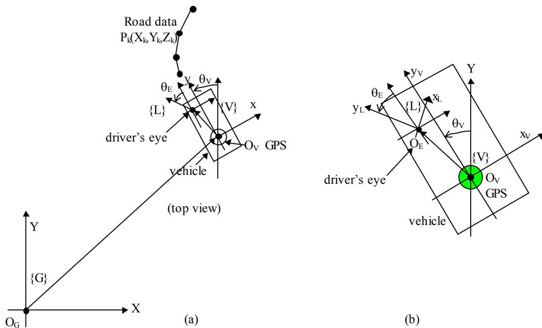
**Figure 27. Coordinate frames used to determine the transformation matrix  $[T]$ .
