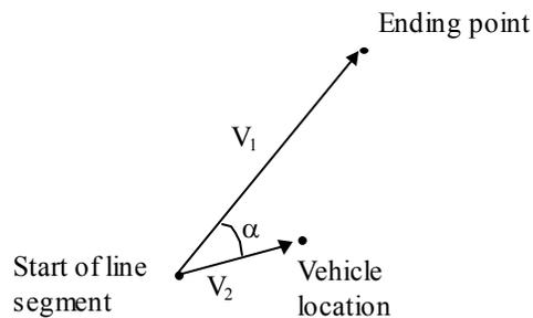
**Figure 39. Vectors for finding the vehicle location with respect to the centerline.**
