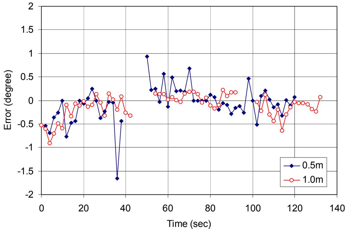
**Figure 60. Effect on error or *vsa* of look-back distances 0.5m and 1.0m at 10mph.**
