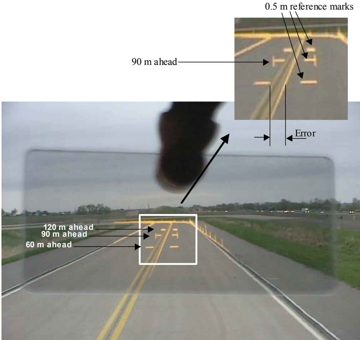
**Figure 51. Reference marks for error analysis (blown up from the central portion of the Figure 50).**
