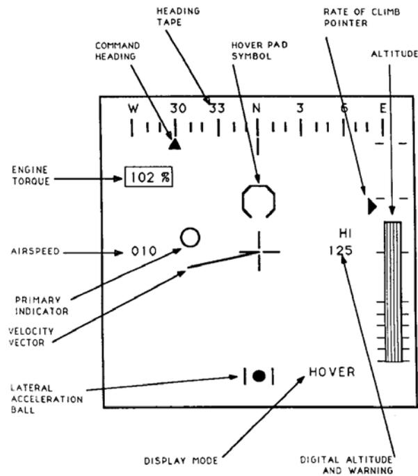
**Figure 6. Position-velocity-acceleration display format.**
