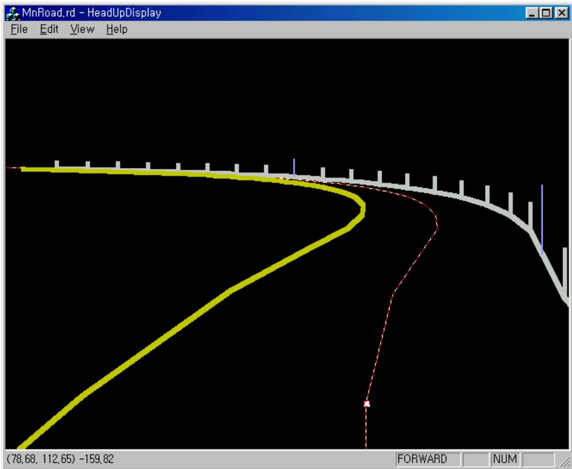
**Figure 21. Typical HUD Screen. The image is in color on a standard display and monochrome in the HUD combiner.**
