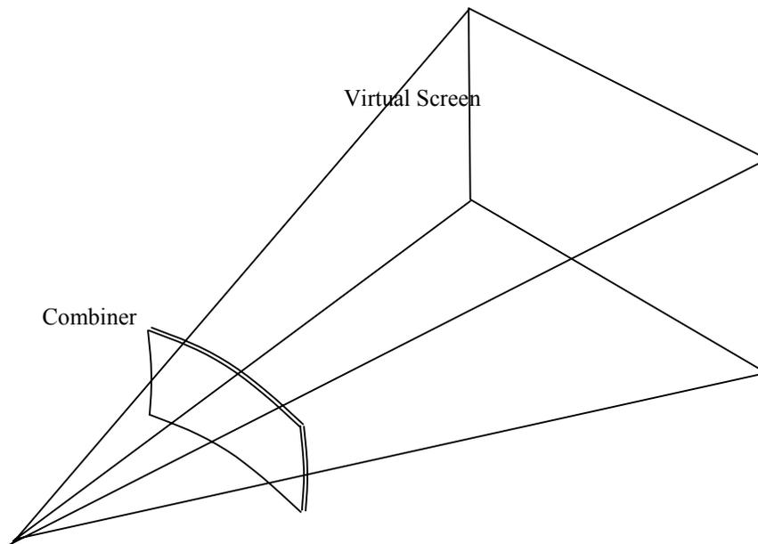
**Figure 12. The virtual screen composed by the combiner.**
