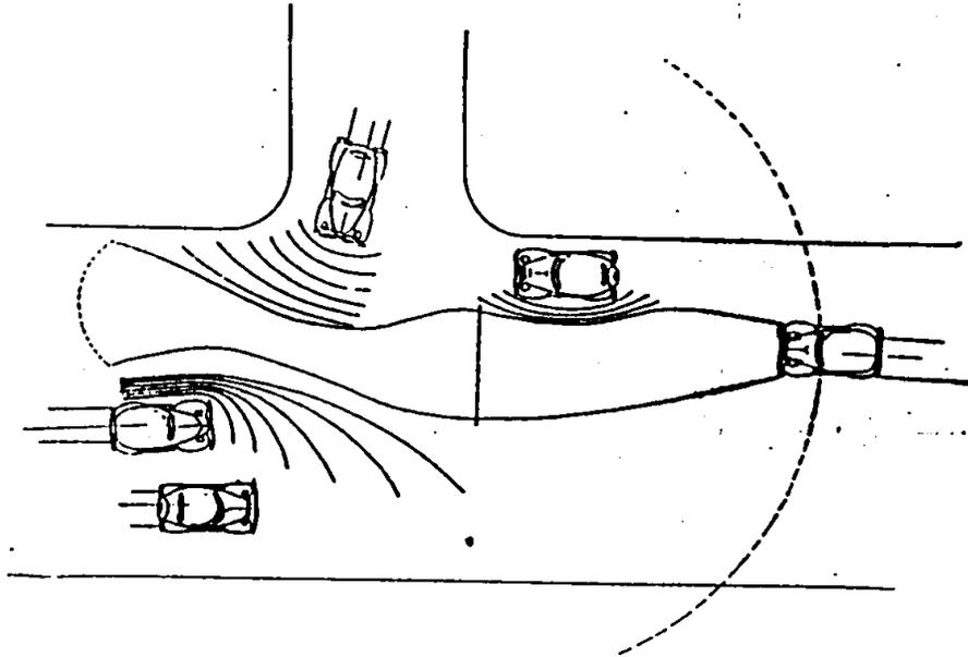
**Figure 2. The field of safe travel and the minimum stopping zone of a driver in traffic.**
