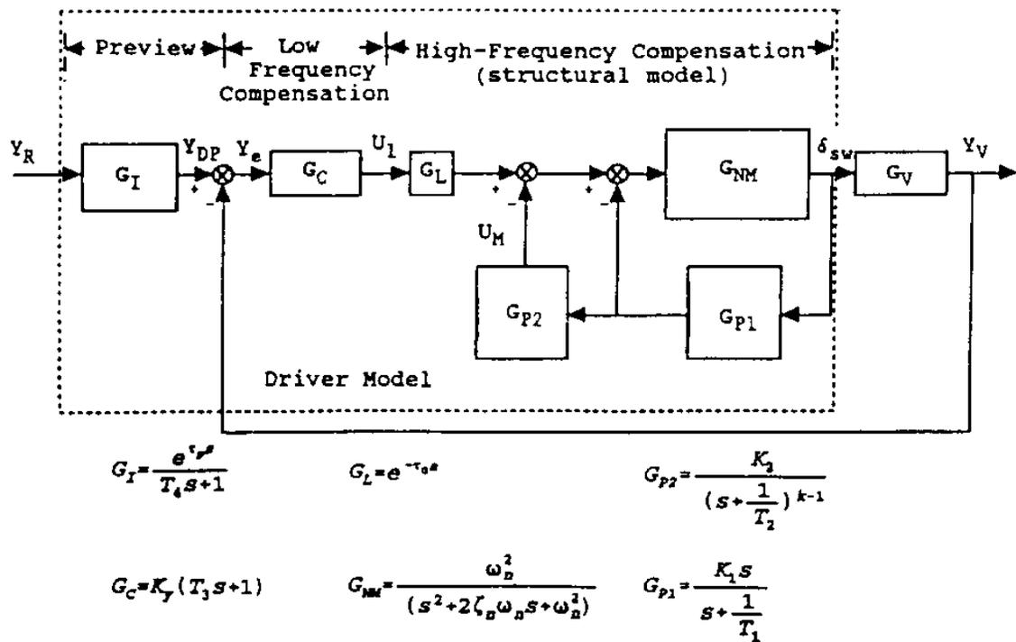
Figure 3. Driver/vehicle control model, Modjtahedzadeh and Hess 1993
