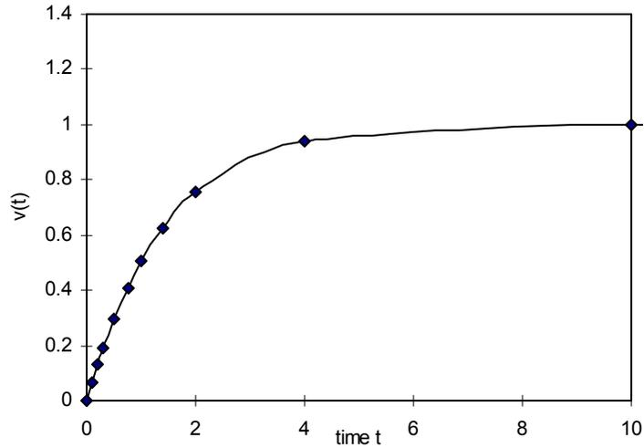
**Figure 41. Velocity profile of the 1st order system**
