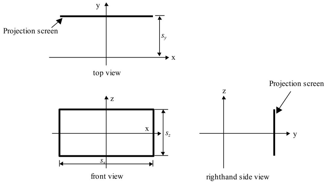
**Figure 31. Geometric diagram of the projection screen.**
