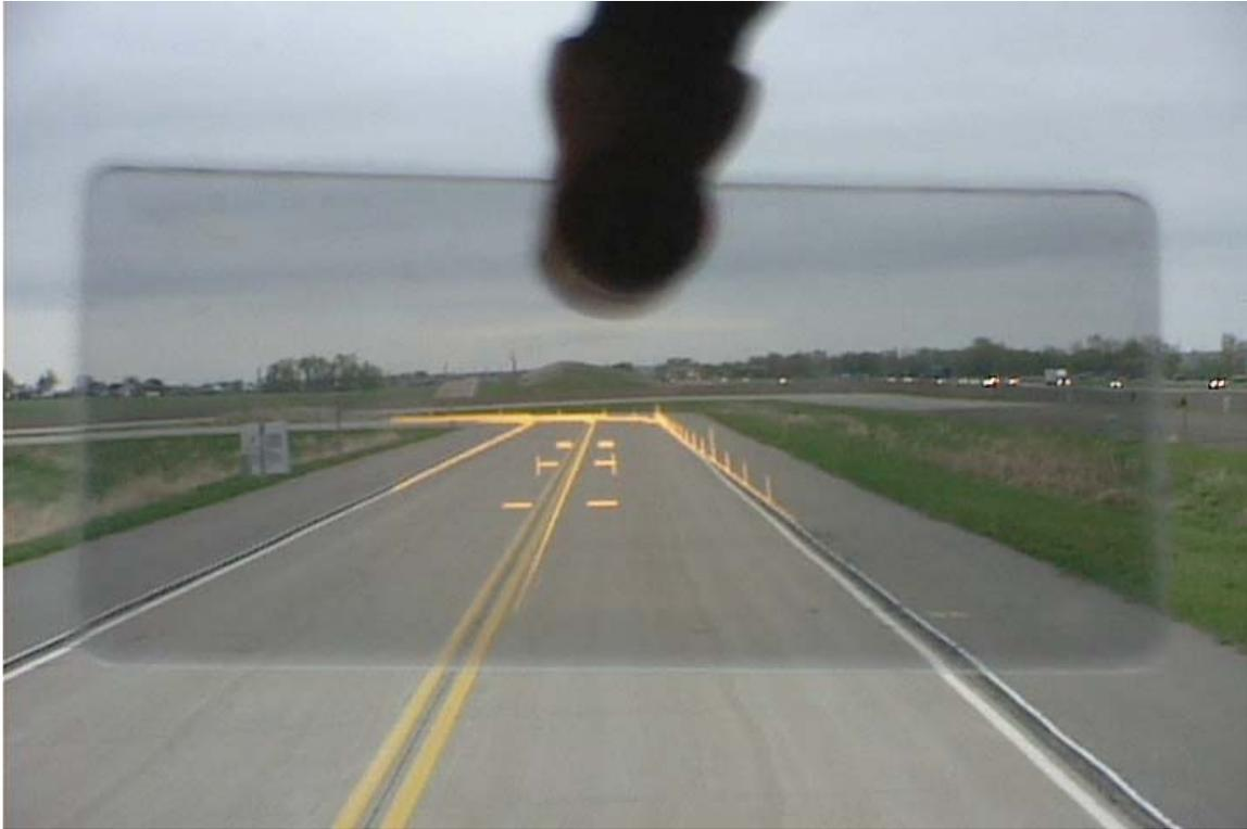
**Figure 50. Typical driving situation with the HUD combiner.**
