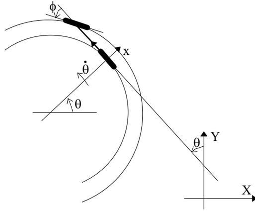
**Figure 43. The changing rate of the heading angle with respect to the steering angle.**
