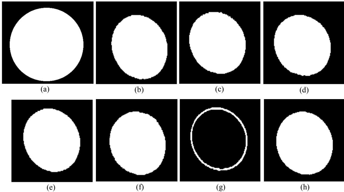
**Figure 56. Calibration image for the optical system of the HUD. (a) A perfect circle image stored in the computer graphic memory, (b,c,d,e,f,g,h) Images of the circle projected on the virtual screen of the HUD system and captured by digital camera.**
