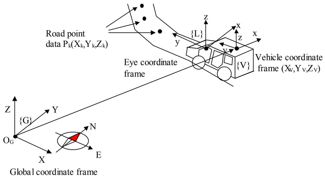
**Figure 23. Coordinate frames (global, vehicle, and local coordinate frames).**
