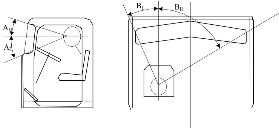
**Figure 19. Field of view through the full windshield.**
