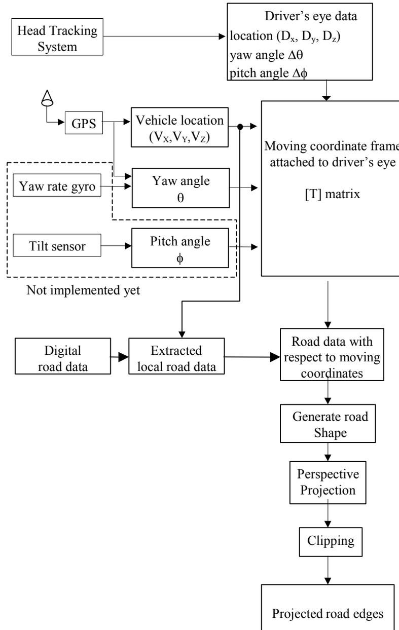
Figure 22. Block diagram of the Head Up Display System.
