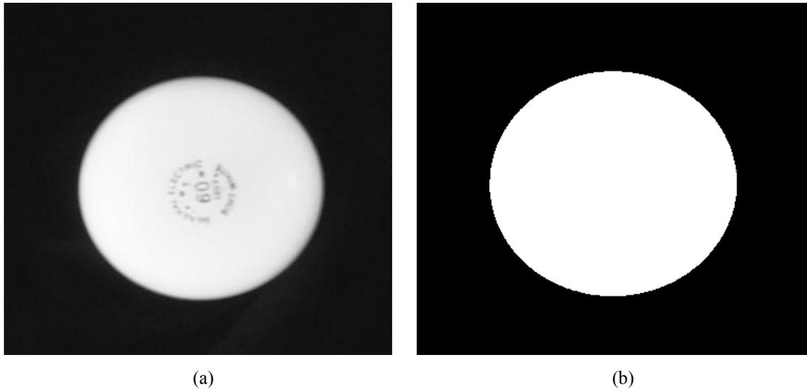
**Figure 55. Light bulb used for calibration of the video camera and the digital image acquisition system. (a) Grayscale image of a soft white light bulb, (b) Binary image of the image (a)**
