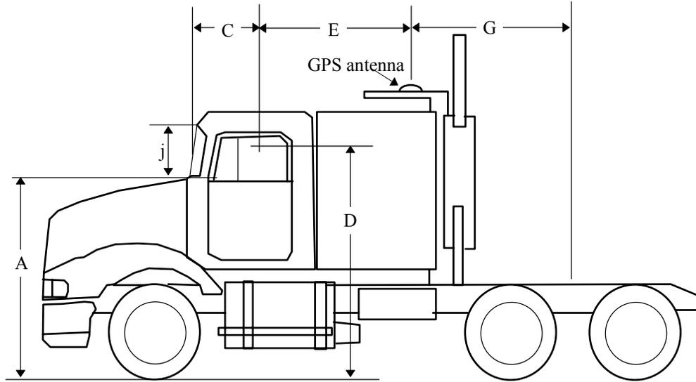
**Figure 18. External dimensions of the truck.**
