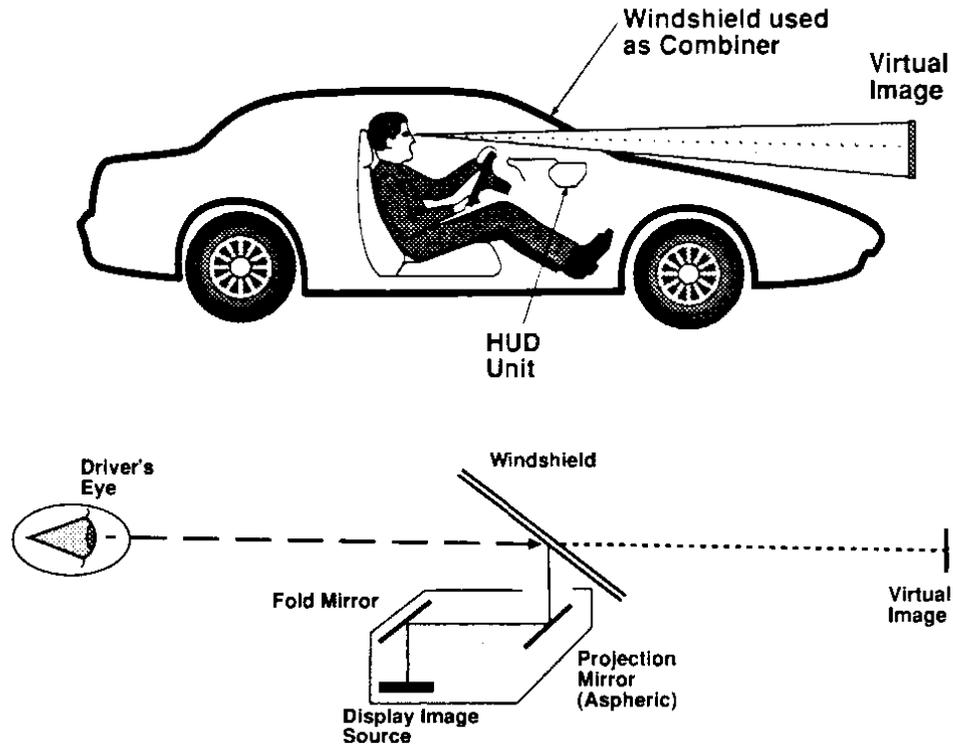
**Figure 7. The first automotive head up display introduced by General Motors.**
