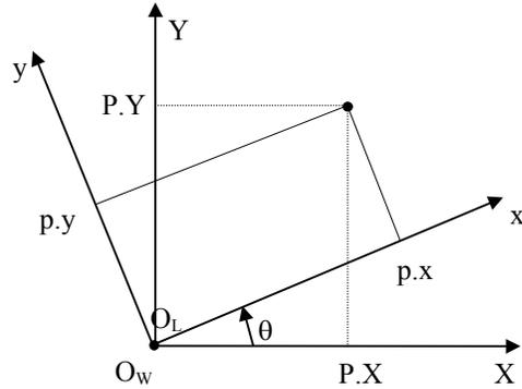
**Figure 29. Rotation of the coordinate frame (P: world coordinates, p: local coordinates).**
