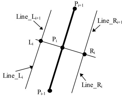
**Figure 26. The case when 2 lines are parallel to each other, i.e. the determinant of  $[M]$  is zero.**
