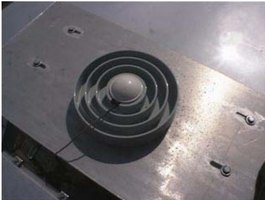
**Figure 20. DGPS receiver antenna mounted on the top of the test truck within a choke ring.**
