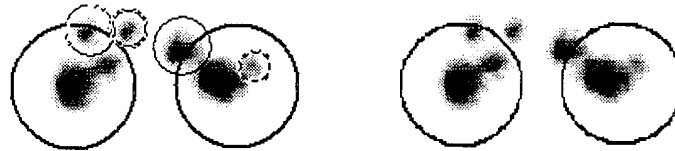
Figure 12: Example of Hough blobs and pairing compared with positional blob finding.
