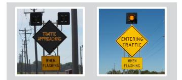
**Intersection Conflict Warning System (ICWS)** have dynamic flashing signs and detection that provide active warning about traffic on the major road, minor road, or both roads at the intersection.
