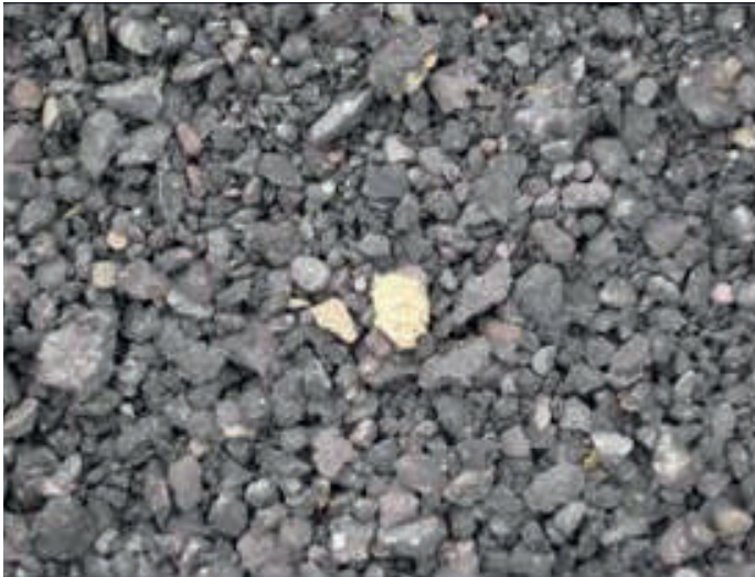
Example of crushed Recycled Asphalt Pavement (RAP) Material
