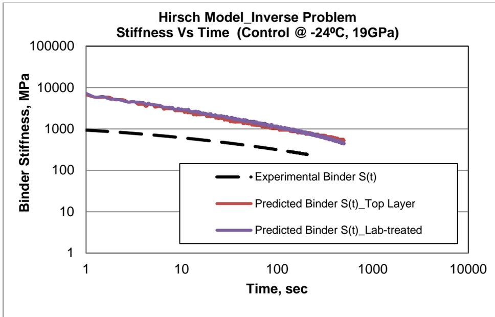
FIGURE 6.24 Hirsch Model Using  $E_{agg}=19$  GPa for Control Mixture Section.
