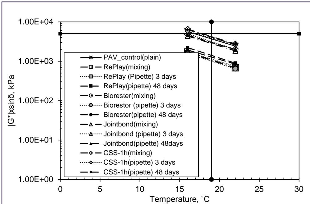
**FIGURE 4.12 PAV  $|G^*|/\sin \delta$  Results at 19°C.**
