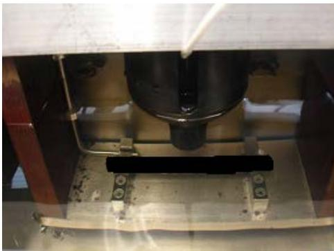
**FIGURE 3.1 BBR Testing Setup for Binders.**
