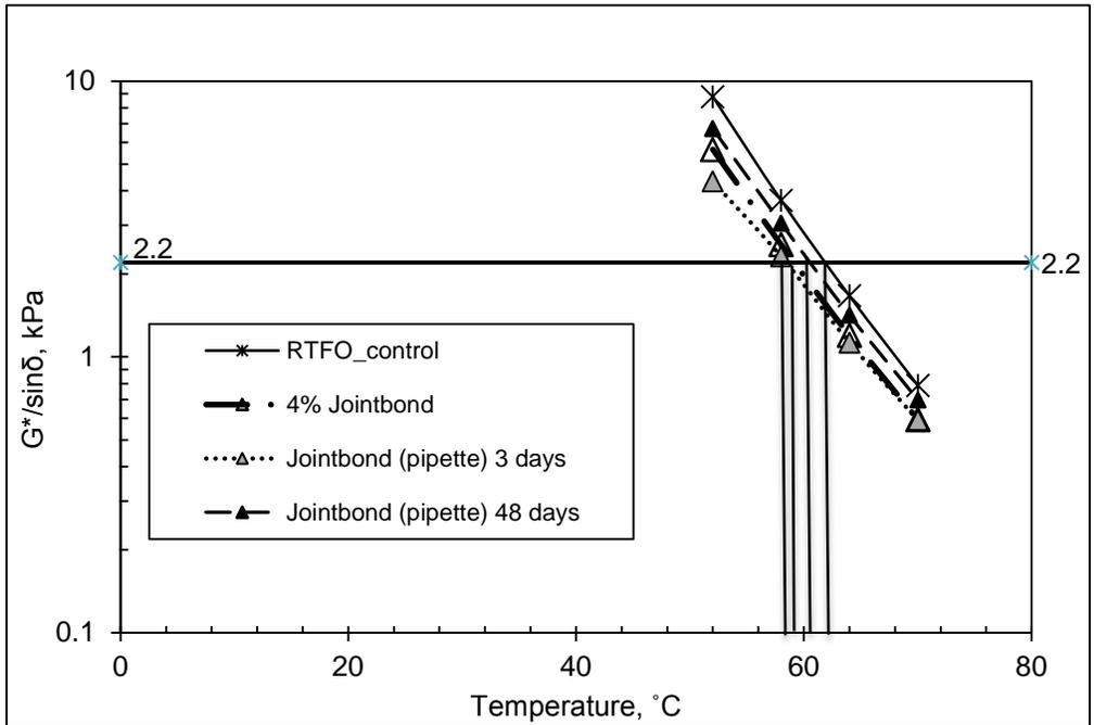
**FIGURE 6.3** Change in Rutting Factor of Binder Treated with Jointbond due to Different Application Process and Storage Time.
