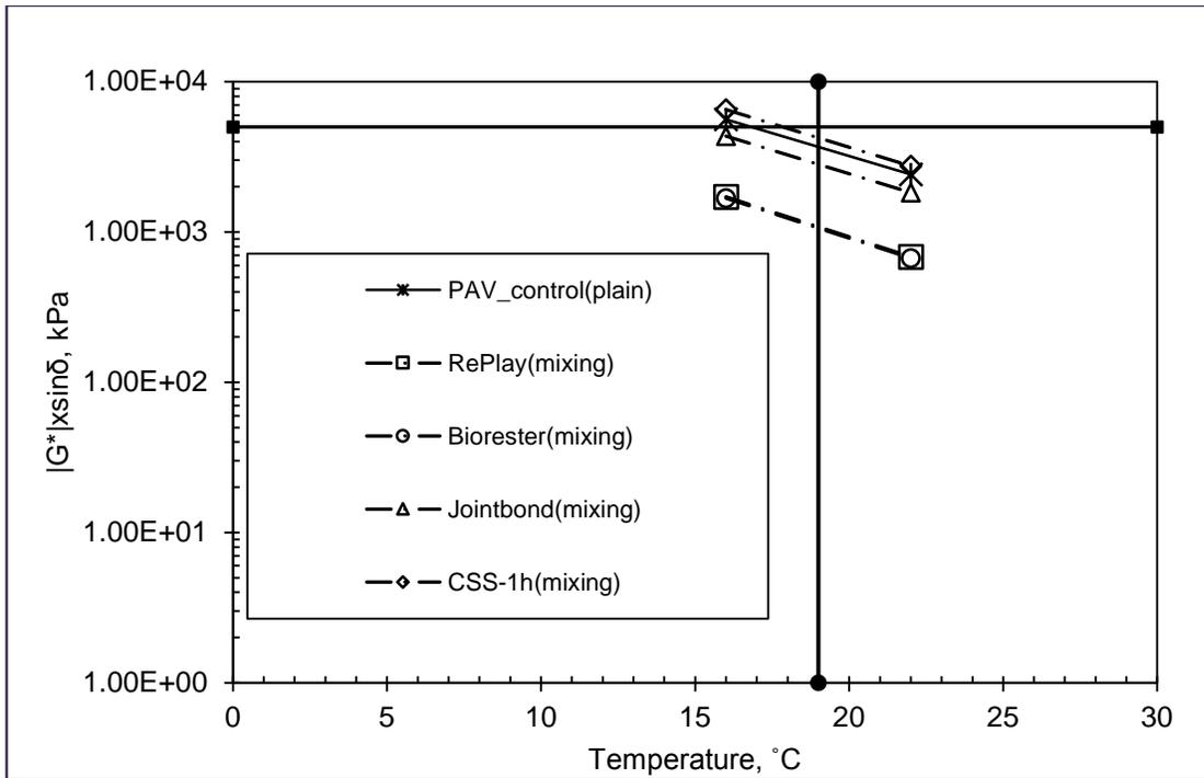
**FIGURE 6.6** Change in Fatigue Factor due to Mixing Method.
