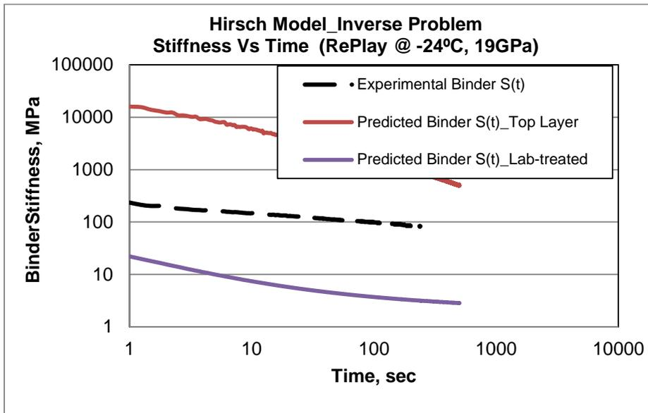
FIGURE 6.25 Hirsch Model Using  $E_{agg}=19$  GPa for Mixture Treated with RePlay.
