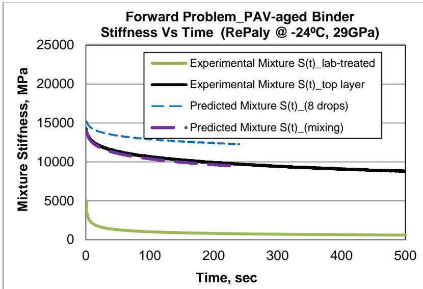
**FIGURE A.7 Hirsch Model using  $E_{agg}=29$  GPa for PAV-aged PG 58-28 Treated with RePlay.**
