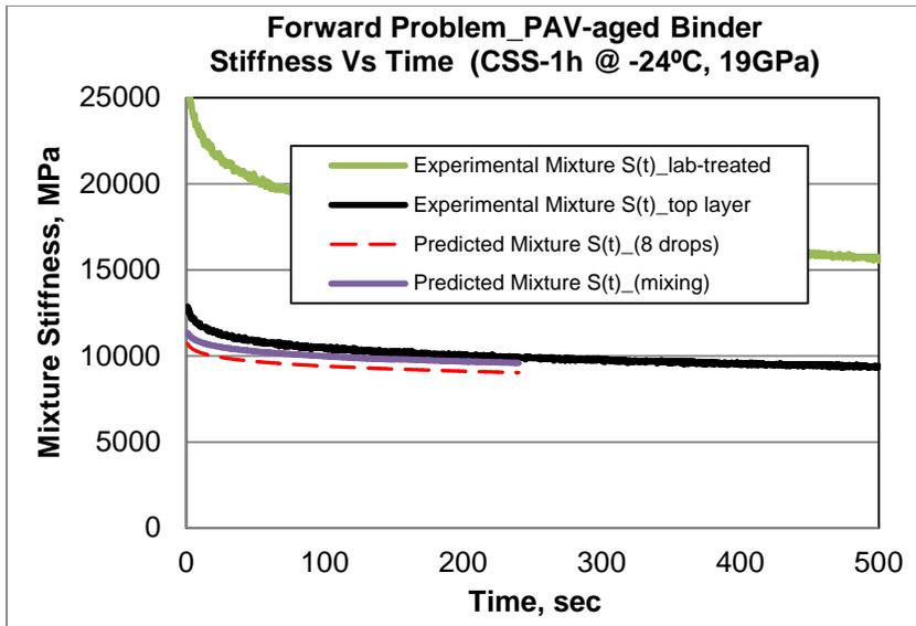
**FIGURE A. 5 Hirsch Model using  $E_{agg}=19$  GPa for PAV-aged PG 58-28 Treated with CSS-1h.**
