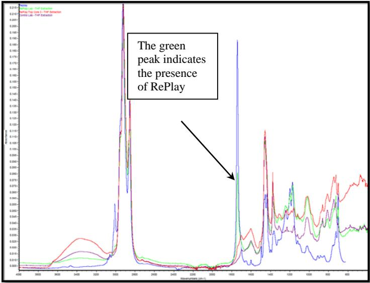
**FIGURE 6.11** Stacked absorbance spectra for RePlay and RePlay treated samples.
