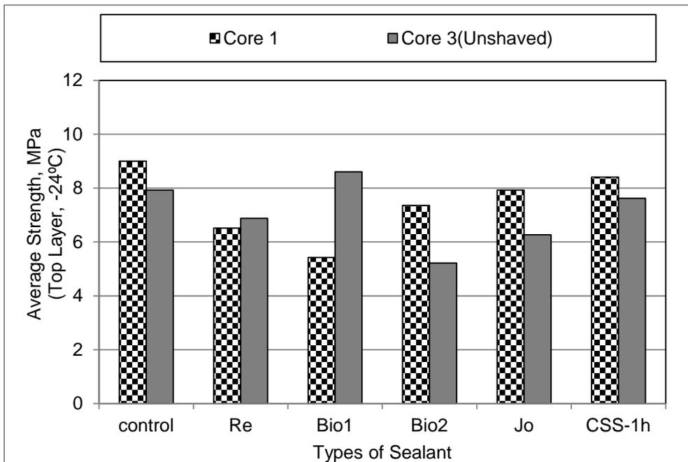
**FIGURE 5.26 Average Strength of Mixture Beams for Shaved and Unshaved Top Surface at -24°C.**
