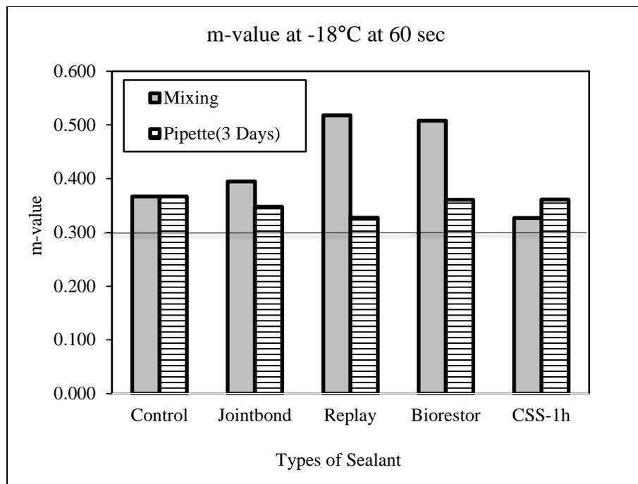
**FIGURE 4.16 PAV  $m(60s)$  Results at  $-18^{\circ}\text{C}$ .**
