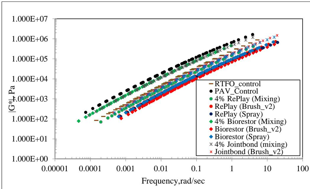
**FIGURE 4.10 DSR Master Curve (Large Plate) of PAV-aged PG 58-28 for Three Different Procedures.**
