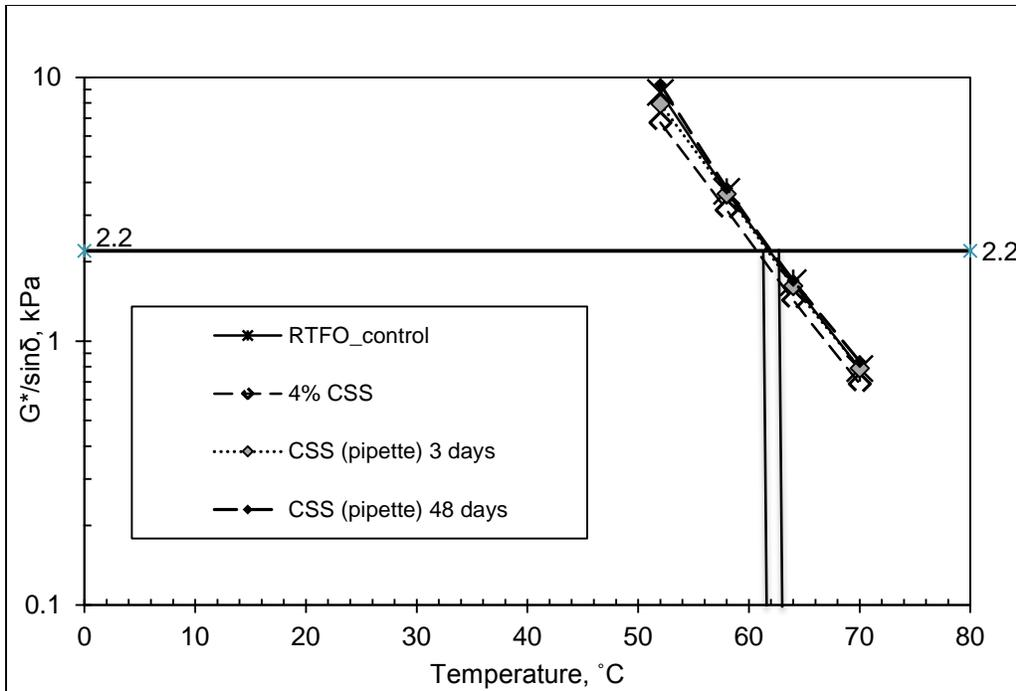
**FIGURE 6.4** Change in Rutting Factor of Binder Treated with CSS-1h due to Different Application Process and Storage Time.
