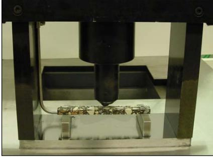
**FIGURE 3.2** *Bending Beam Rheometer with thin asphalt mixture (28).*
