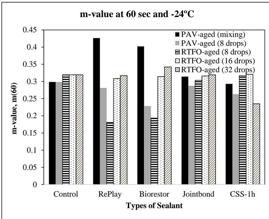
**FIGURE 4.18** Change in m-value due to PAV-aging, RTFOT-aging and Different Application Rate of the Sealant.
