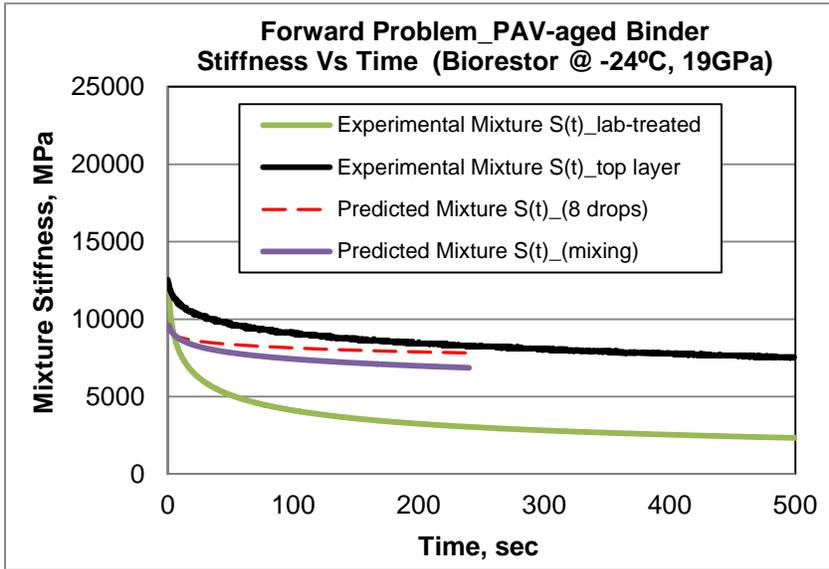
**FIGURE A.3 Hirsch Model using  $E_{agg}=19$  GPa for PAV-aged PG 58-28 Treated with Biorestor.**
