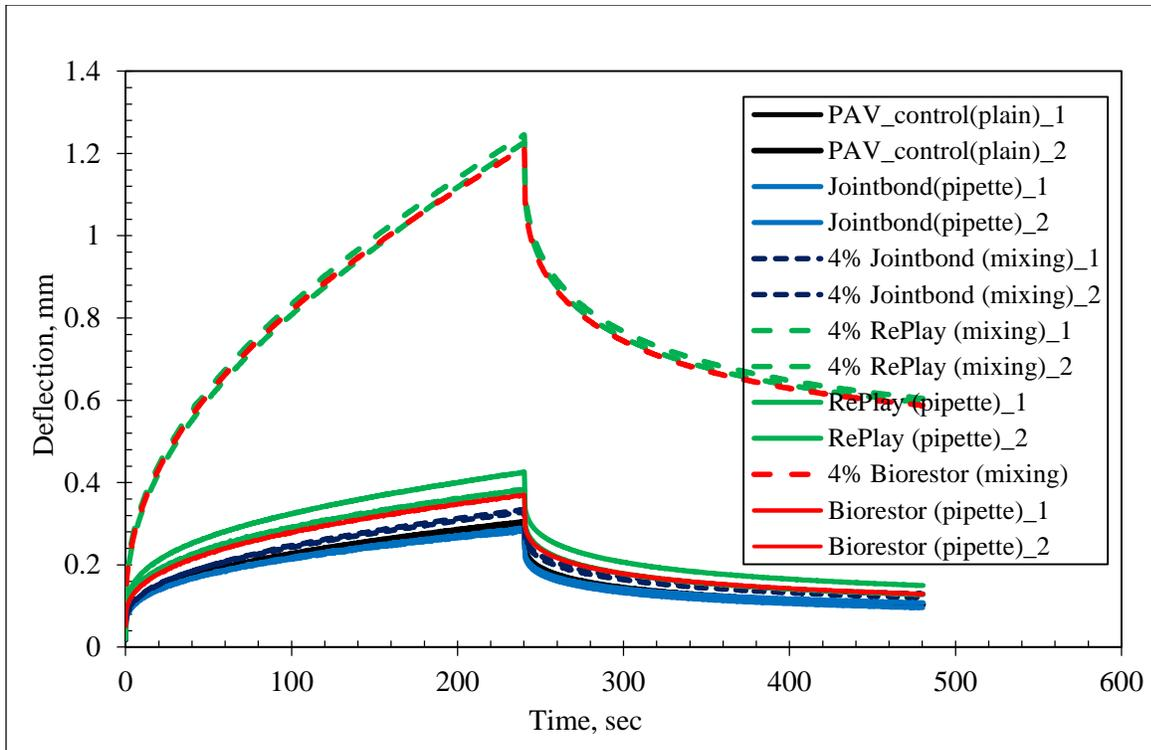
**FIGURE 4.14** Deflection vs Time for PAV-aged PG 58-28 at -24°C.
