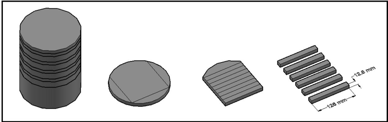
**FIGURE 3.3** *Asphalt Mixture Beam Preparation (28).*
