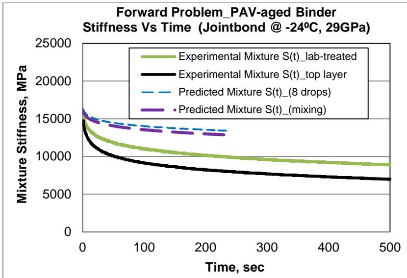
**FIGURE A.9 Hirsch Model using  $E_{agg}=29$  GPa for PAV-aged PG 58-28 Treated with Jointbond.**
