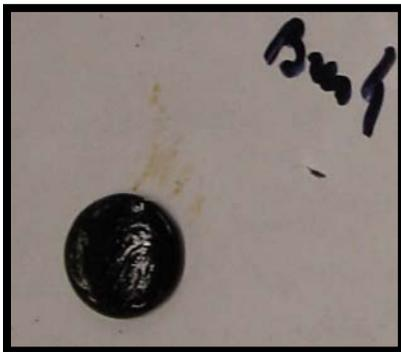
**FIGURE 4.3 DSR large plate specimen after 72 hours from brushing.**
