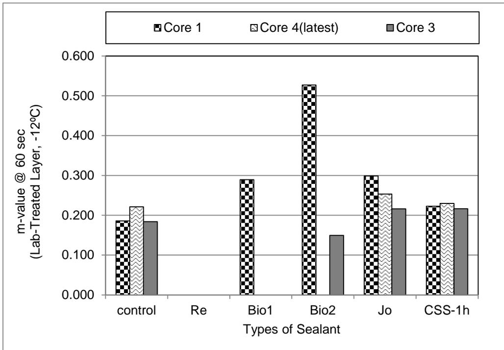
**FIGURE 5.12** *m-value(60s) Results at -12°C of Mixture Beams from Lab-Treated Layer.*
