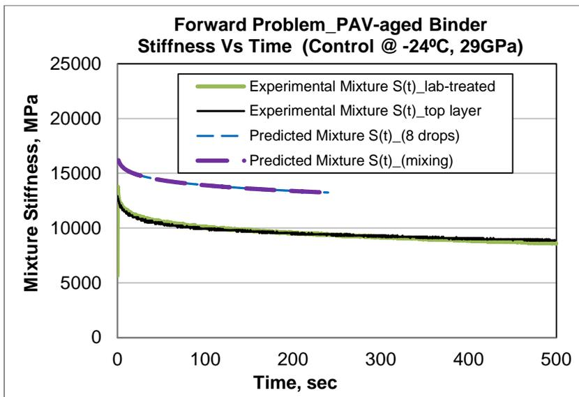
**FIGURE A.6 Hirsch Model using  $E_{agg}=29$  GPa for Control PAV-aged PG 58-28.**
