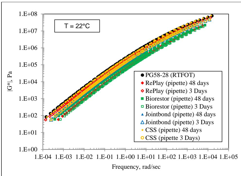
**FIGURE 4.7**  $|G^*|$  Master Curves for RTFOT and Pipette Method.
