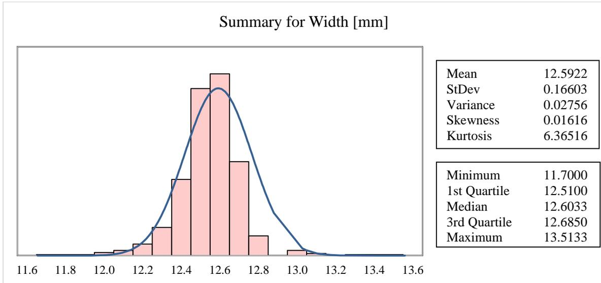
**FIGURE 5.2 Statistics for BBR Mixture Beams Width.**
