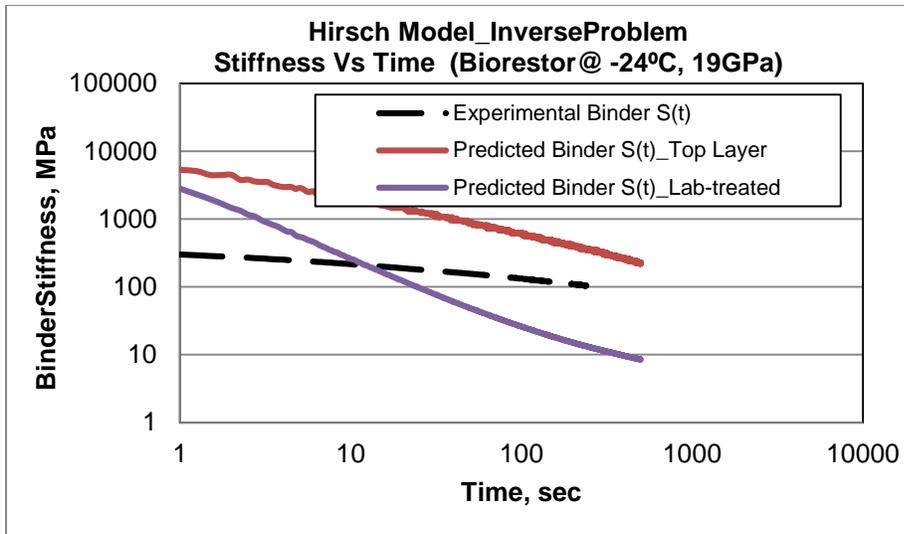
**FIGURE 6. 26 Hirsch Model using  $E_{agg}=19$  GPa for Mixture treated with Biorestor.**
