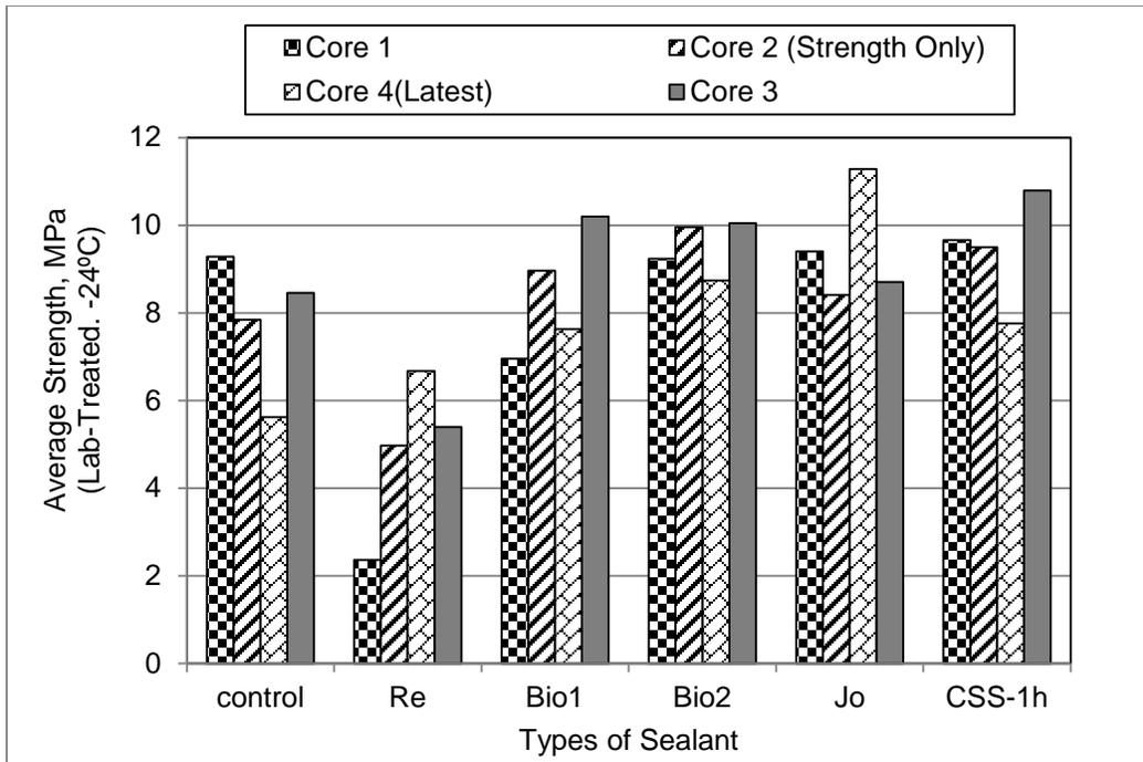
**FIGURE 5.14 Strength at -24°C of Mixture Beams from Lab-Treated Layer.**
