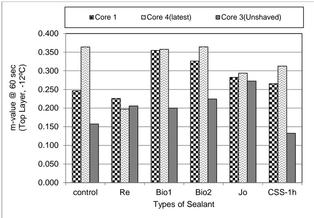
**FIGURE 5.11** *m-value(60s) Results at -12°C of Mixture Beams from Field Treated/Top Layer.*
