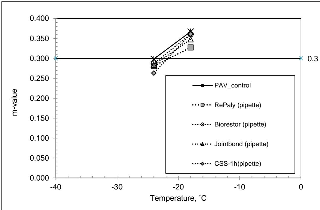
**FIGURE 6.8** Change in *m*-value due to Pipette Method.
