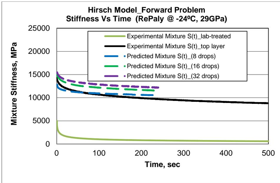
**FIGURE 6.19** Hirsch Model Using  $E_{agg}=29$  GPA for RTFO-aged PG 58-28 Treated with RePlay.
