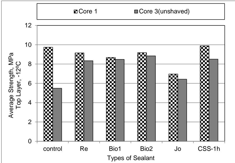
**FIGURE 5.25 Average Strength of Mixture Beams for Shaved and Unshaved Top Surface at -12°C.**
