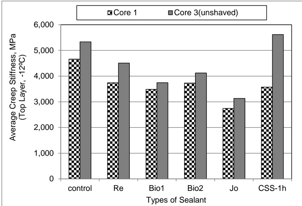
**FIGURE 5.21** Creep Stiffness of Mixture Beams for Shaved and Unshaved Top Surface at -12°C.
