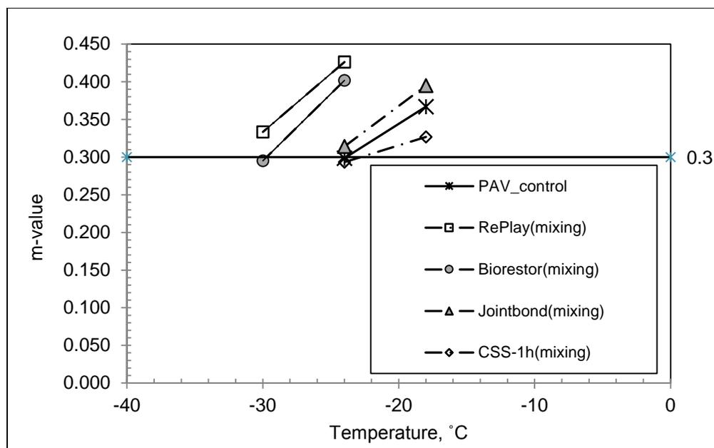
**FIGURE 6.10** Change in *m*-value due to Mixing Method.
