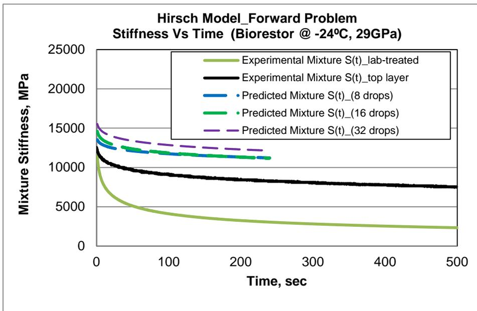
**FIGURE 6.20** Hirsch Model Using  $E_{agg}=29$  GPA for RTFO-aged PG 58-28 Treated with Biorestor.
