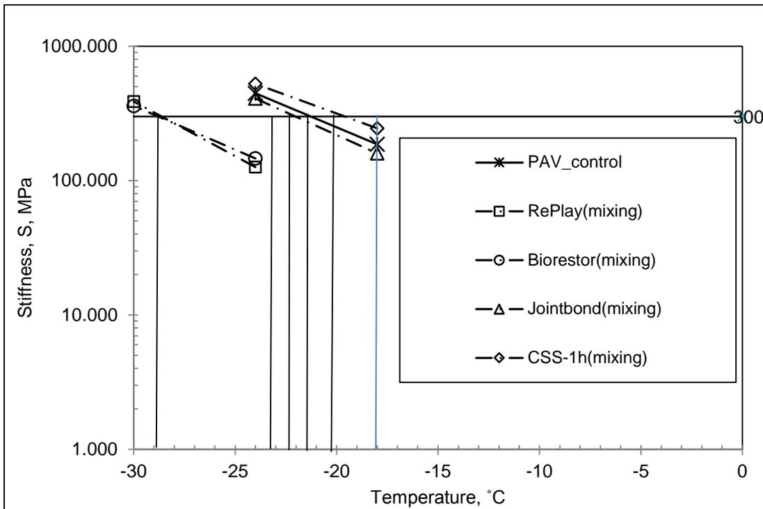
**FIGURE 6.9** Change in Creep Stiffness due to Mixing Method.
