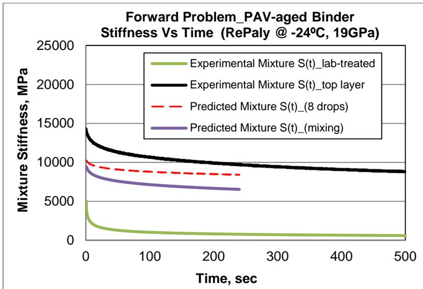
**FIGURE A. 2** Hirsch Model using  $E_{agg}=19$  GPa for PAV-aged PG 58-28 Treated with RePlay.
