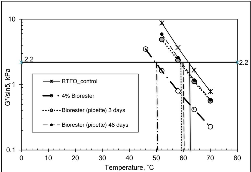
**FIGURE 6.2** Change in Rutting Factor of Binder Treated with Biorester due to Different Application Process and Storage Time.
