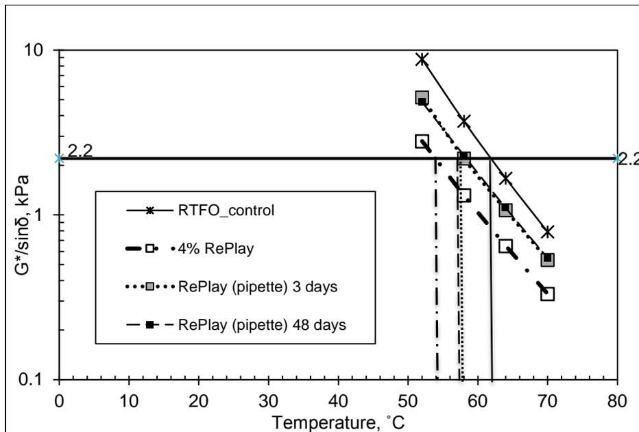
**FIGURE 6.1** Change in Rutting Factor of Binder Treated with RePlay due to Different Application Process and Storage Time.
