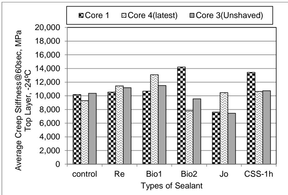
**FIGURE 5.5 S(60s) Results at -24°C of Mixture Beams from Field Treated/Top Layer.**
