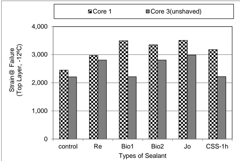
**FIGURE 5.27  $\mu$ Strain at Failure of Mixture Beams for Shaved and Unshaved Top Surface at  $-12^{\circ}\text{C}$ .**
