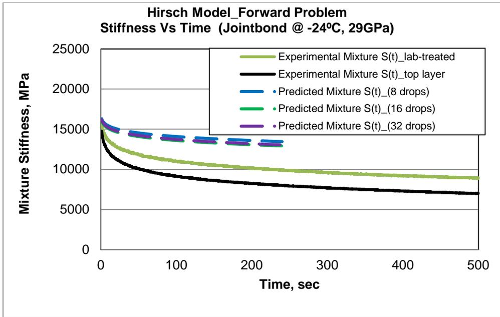
**FIGURE 6.21** Hirsch Model Using  $E_{agg}=29$  GPa for RTFO-aged PG 58-28 Treated with Jointbond.
