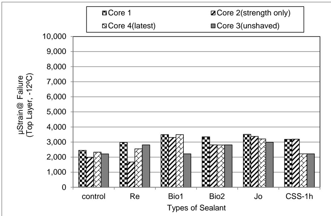
**FIGURE 5.19** *μStrain at Failure at -12°C of Mixture Beams from Field Treated/Top Layer.*
