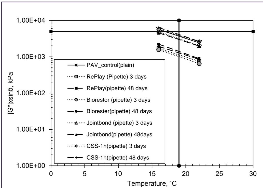
**FIGURE 6.5** Change in Fatigue Factor due to Pipette method.
