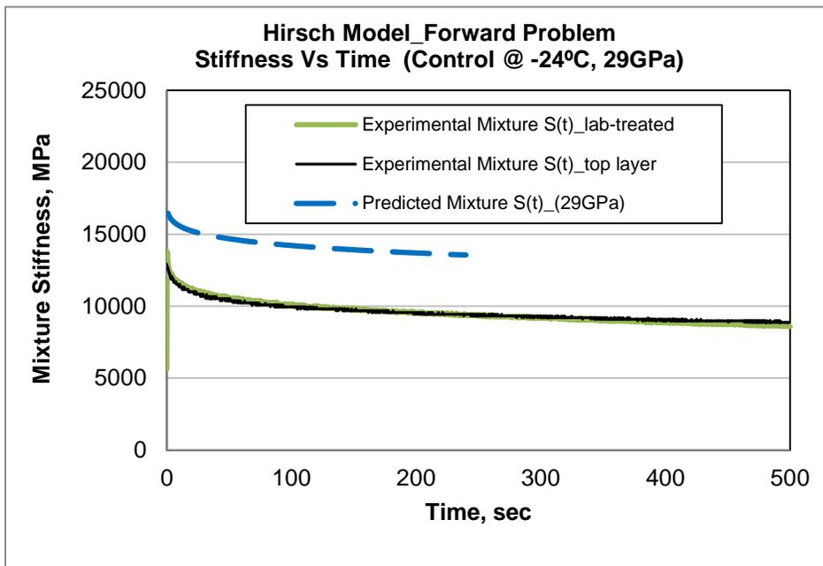
**FIGURE 6.18** Hirsch Model using  $E_{agg}=29$  GPa for control RTFO-aged PG 58-28.
