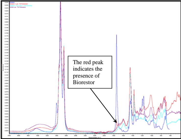
**FIGURE 6.12** Stacked absorbance spectra for Bioestor and Bioestor treated samples.
