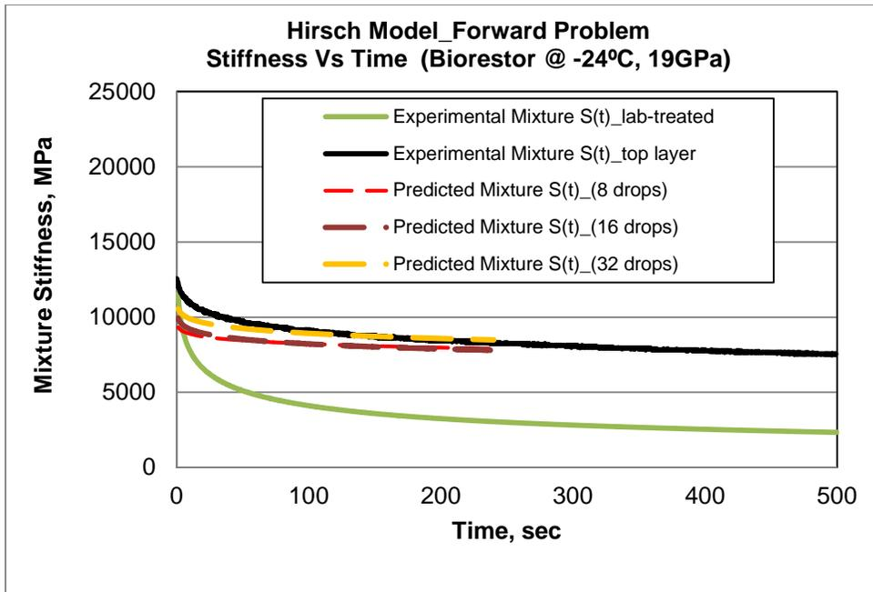
**FIGURE 6.15** Hirsch Model Using  $E_{agg}=19$  GPA for RTFO-aged PG 58-28 Treated with Biorestor.
