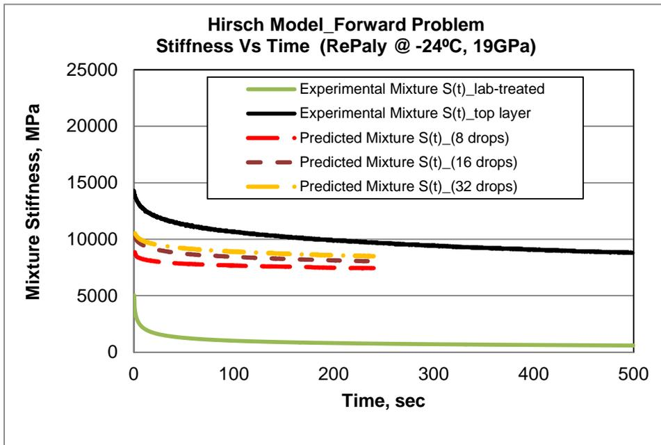
**FIGURE 6.14** Hirsch Model Using  $E_{agg}=19$  GPa for RTFO-aged PG 58-28 Treated with RePlay.
