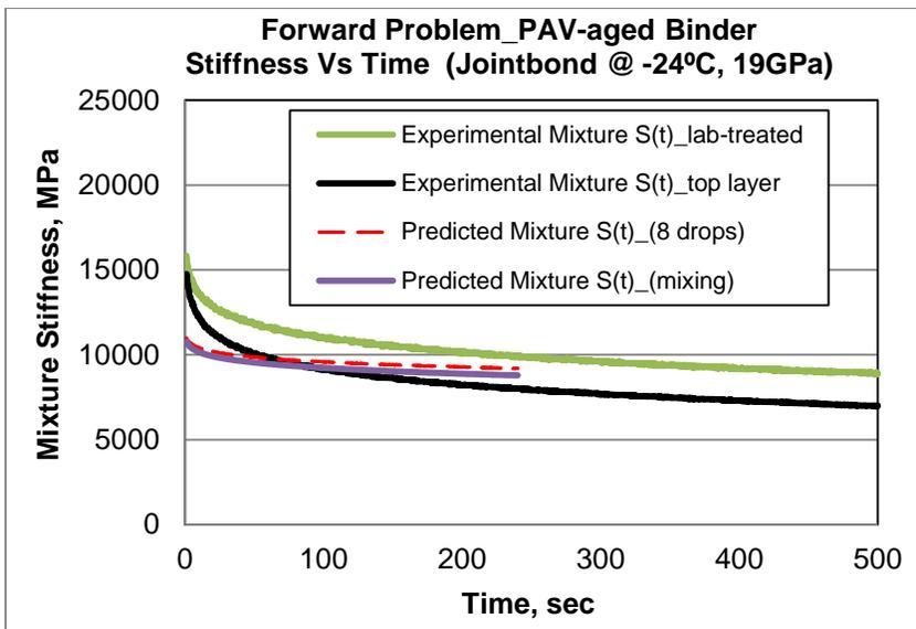
**FIGURE A.4 Hirsch Model using  $E_{agg}=19$  GPa for PAV-aged PG 58-28 Treated with JointBond.**
