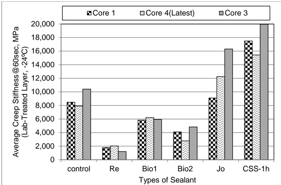
**FIGURE 5.6** *S(60s) Results at -24°C of Mixture Beams from Lab-Treated Layer.*
