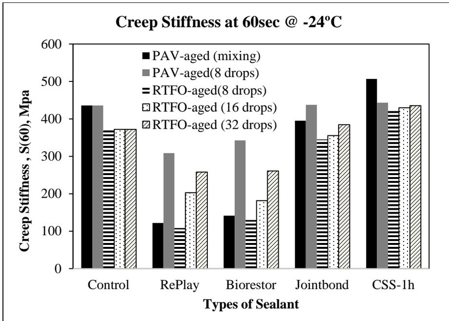
**FIGURE 4.17** Change in Creep Stiffness due to PAV-aging, RTFOT-aging and Different Application Rate of the Sealant.
