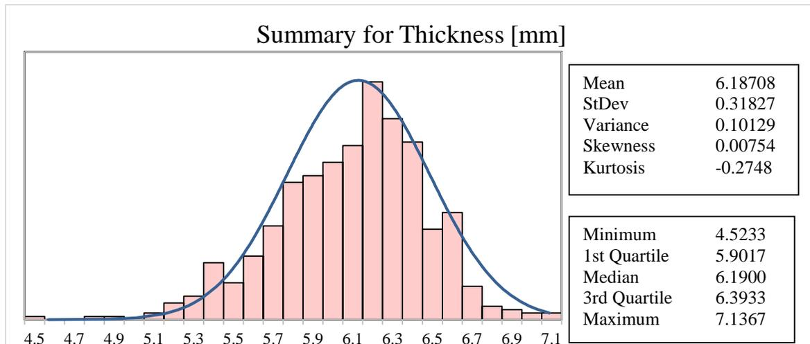
**FIGURE 5.1** Statistics for BBR Mixture Beams Thickness.
