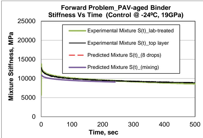
**FIGURE A. 1** Hirsch Model using  $E_{agg}=19$  GPa for Control PAV-aged PG 58-28.
