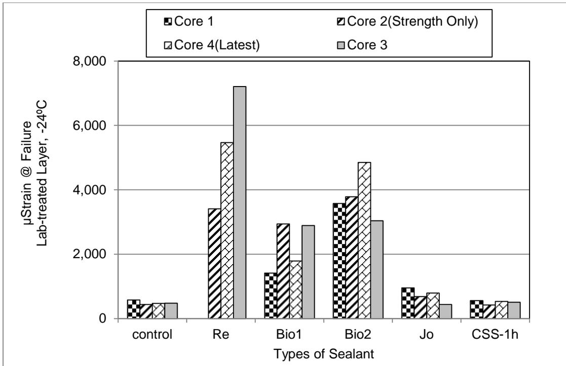
**FIGURE 5.18** *μStrain at Failure at -24°C of Mixture Beams from Lab-Treated Layer.*
