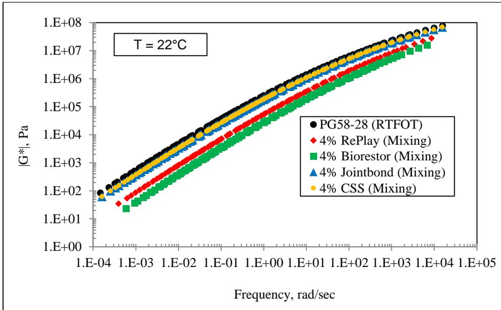
**FIGURE 4.6**  $|G^*|$  Master Curves for RTFOT and Simple Mixing Procedure.
