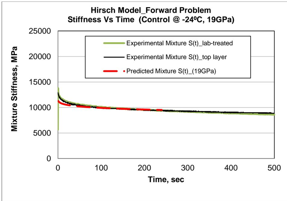
**FIGURE 6.13** Hirsch Model using  $E_{agg}=19$  GPa for Control RTFO-aged PG 58-28.
