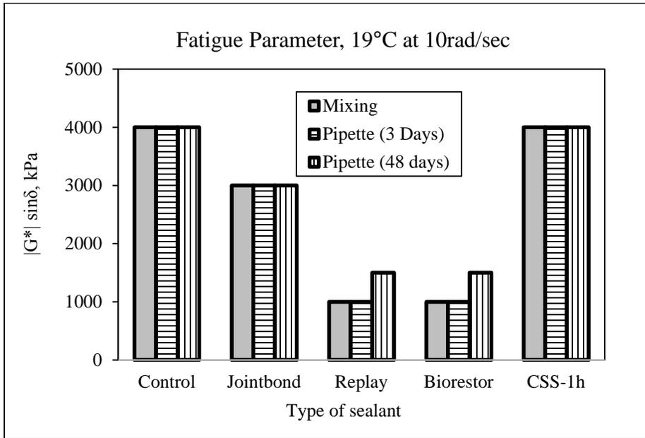
**FIGURE 4.13 PAV  $|G^*| \sin \delta$  Results at 19°C.**
