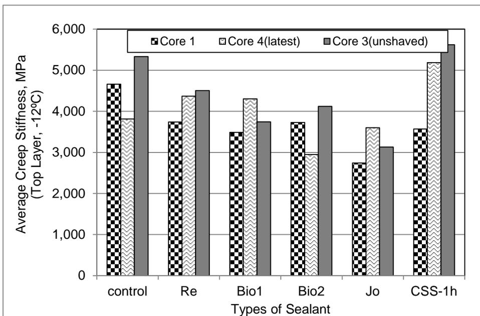
**FIGURE 5.7** *S(60s) Results at -12°C of Mixture Beams from Field Treated/Top Layer.*
