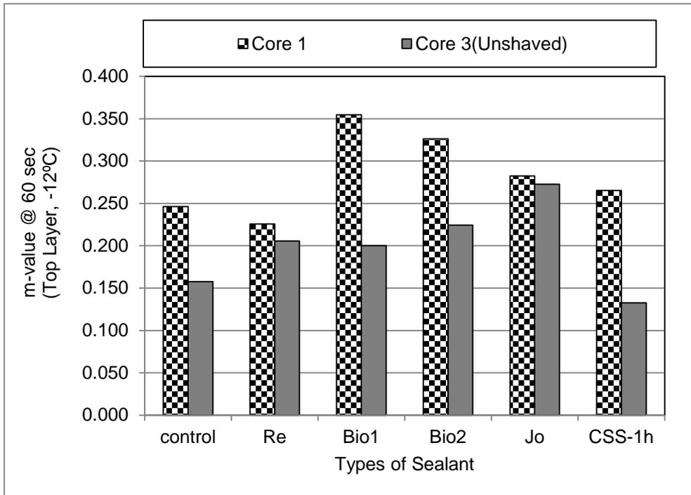
**FIGURE 5.23** m-value of Mixture Beams for Shaved and Unshaved Top Surface at -12°C.
