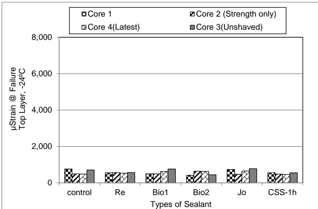
**FIGURE 5.17** μStrain at Failure at -24°C of Mixture Beams from Field Treated/Top Layer.
