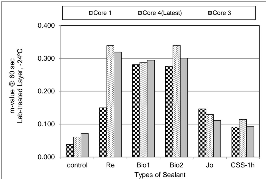
**FIGURE 5.10** *m-value(60s) Results at -24°C of Mixture Beams from Lab-Treated Layer.*
