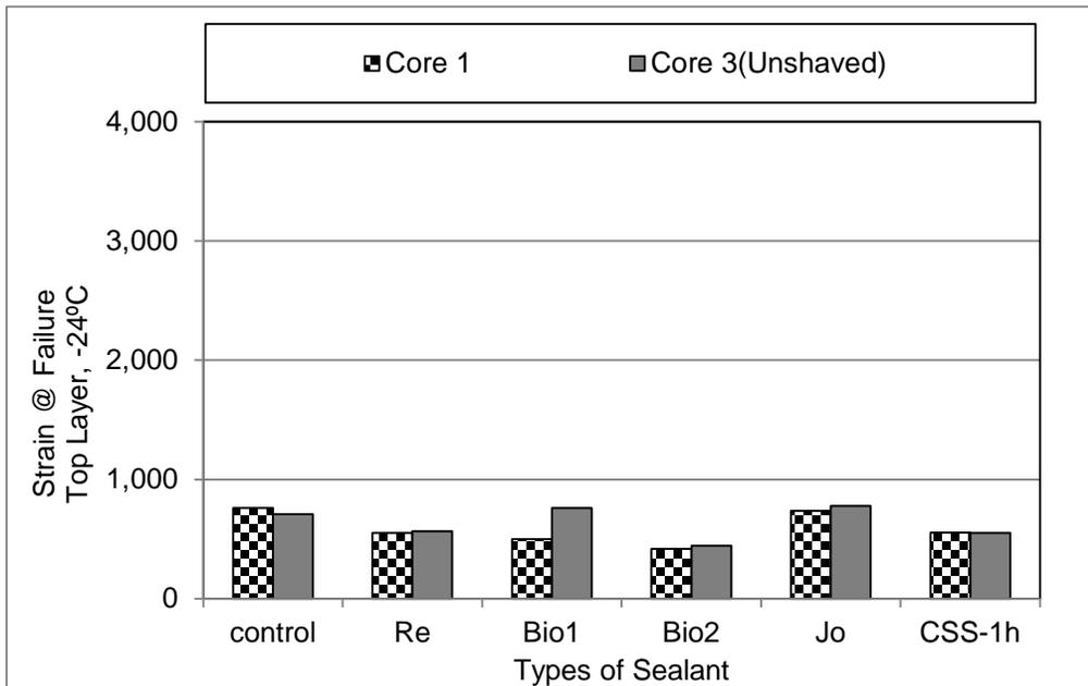
**FIGURE 5.28  $\mu$ Strain at Failure of Mixture Beams for Shaved and Unshaved Top Surface at  $-24^{\circ}\text{C}$ .**
