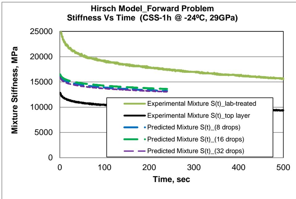
**FIGURE 6.22** Hirsch Model Using  $E_{agg}=29$  GPa for RTFO-aged PG 58-28 Treated with CSS-1h.
