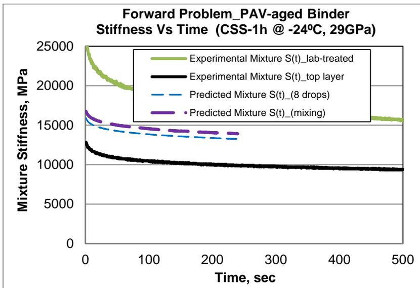
**FIGURE A.10 Hirsch Model using  $E_{agg}=29$  GPa for PAV-aged PG 58-28 Treated with CSS-1h.**
