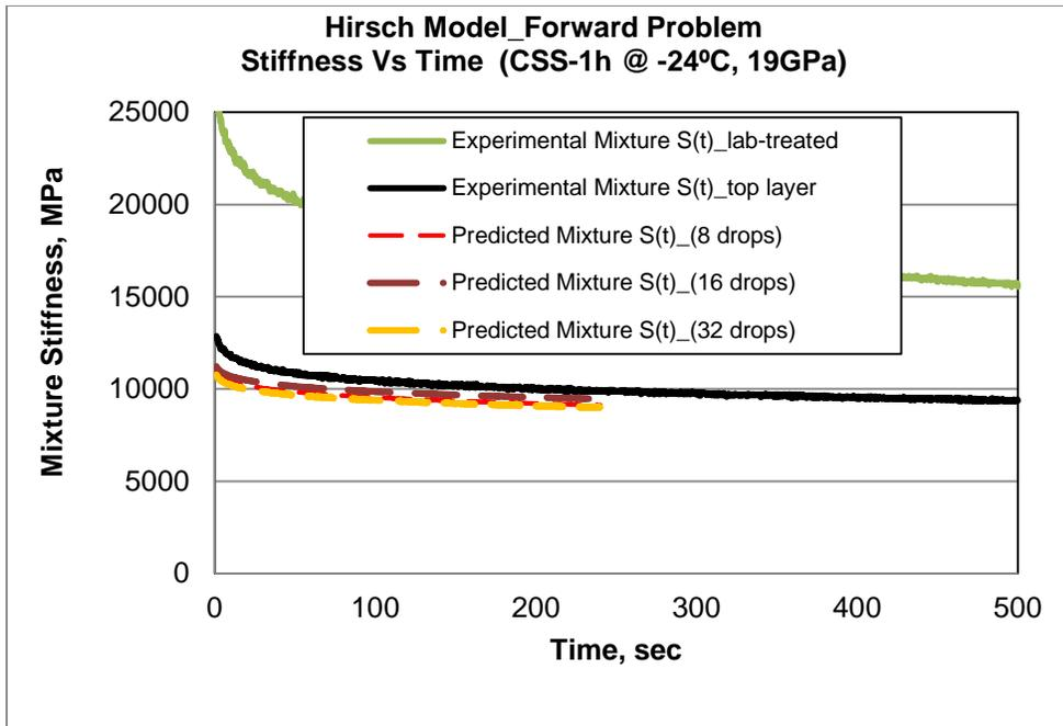
**FIGURE 6.17** Hirsch Model Using  $E_{agg}=19$  GPa for RTFO-aged PG 58-28 Treated with CSS-1h.
