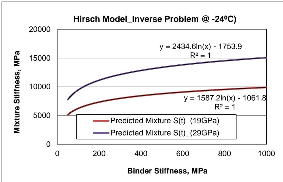
**FIGURE 6.23 Simplified Mixture stiffness function.**
