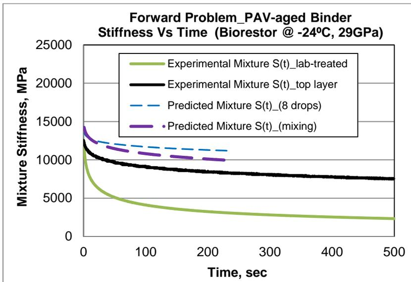
**FIGURE A. 8 Hirsch Model using  $E_{agg}=29$  GPa for PAV-aged PG 58-28 Treated with Biorestor.**
