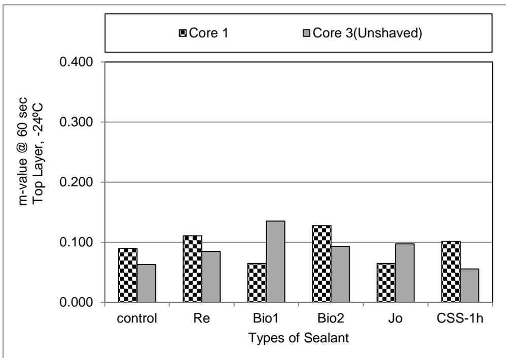
**FIGURE 5.24** m-value of Mixture Beams for Shaved and Unshaved Top Surface at -24°C.
