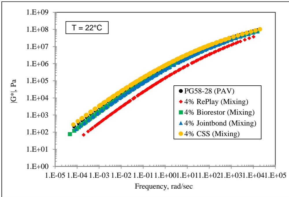
**FIGURE 4.8  $|G^*|$  Master Curves for PAV and Simple Mixing Procedure.**
