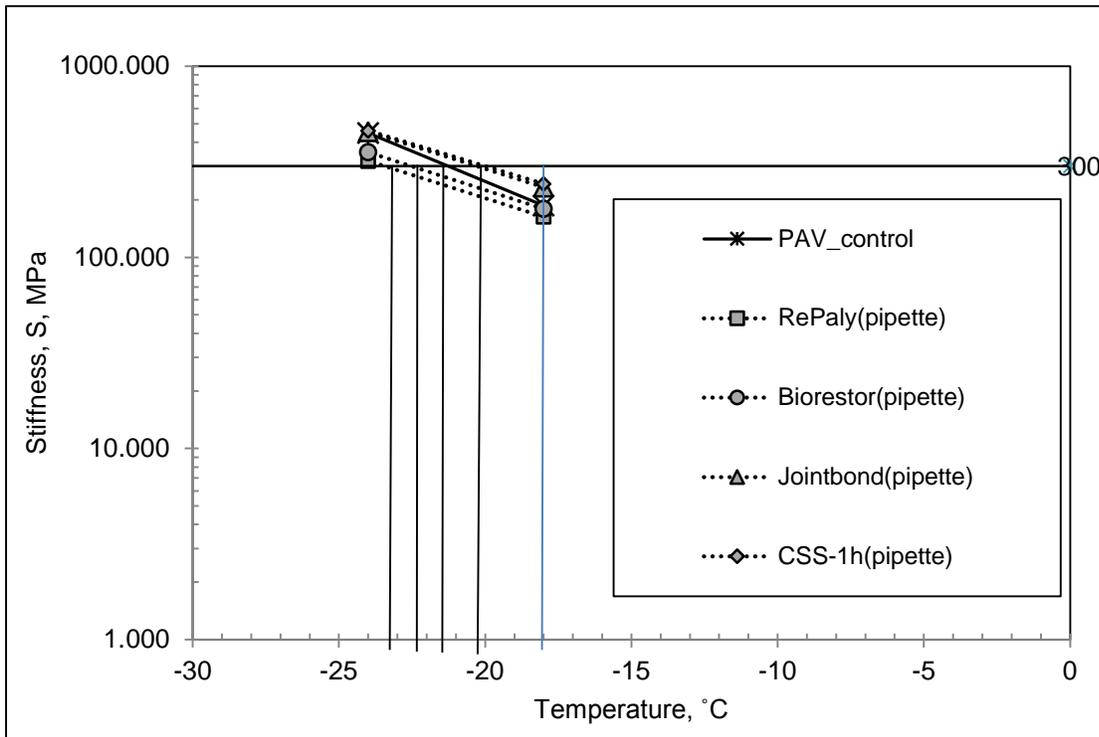
**FIGURE 6.7** Change in Creep Stiffness due to Pipette Method.
