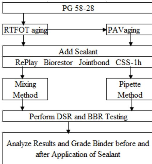
**FIGURE 4.5 Testing Plan of Asphalt Binder.**
