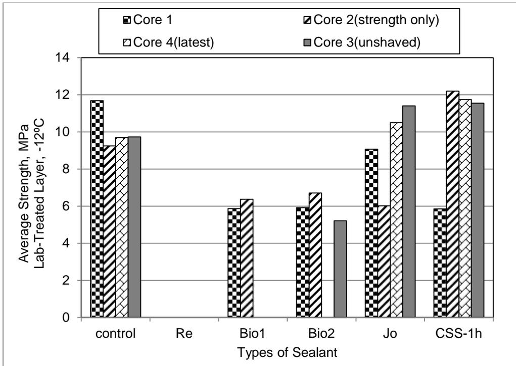
**FIGURE 5.16** Strength at -12°C of Mixture Beams from Lab-Treated Layer.
