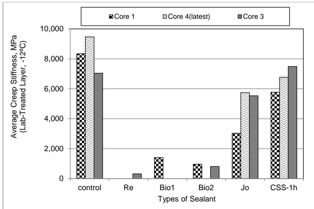
**FIGURE 5.8 S(60s) Results at -12°C of Mixture Beams from Lab-Treated Layer.**
