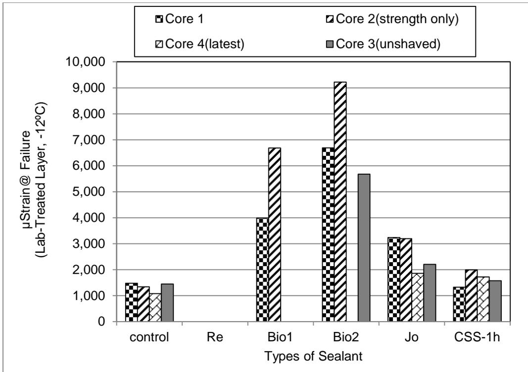
**FIGURE 5.20  $\mu$ Strain at Failure at  $-12^{\circ}\text{C}$  of Mixture Beams from Lab-Treated Layer.**
