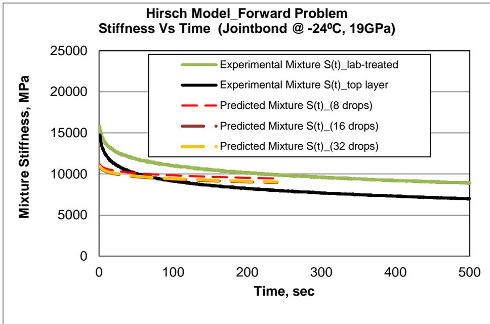
**FIGURE 6.16** Hirsch Model Using  $E_{agg}=19$  GPA for RTFO-aged PG 58-28 Treated with Jointbond.
