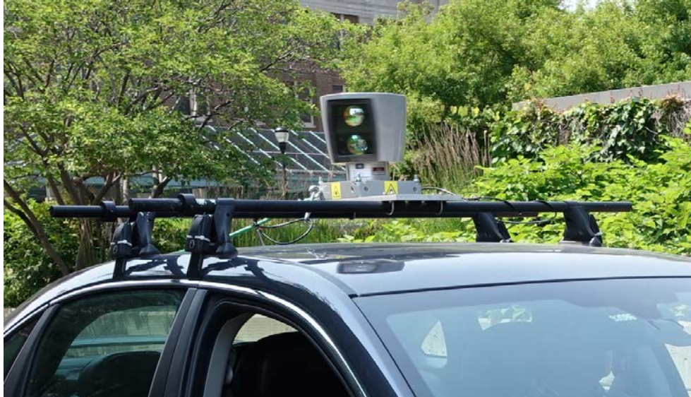
Figure 3.2 Velodyne HDL-64E LIDAR mounted on research vehicle.
