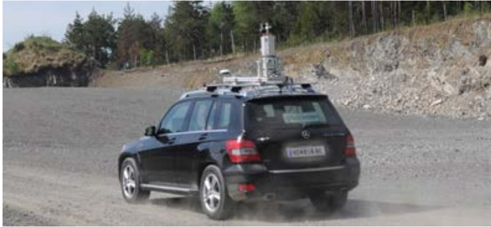
Figure 2.6 Riegl VZ-2000 mounted on a vehicle.
