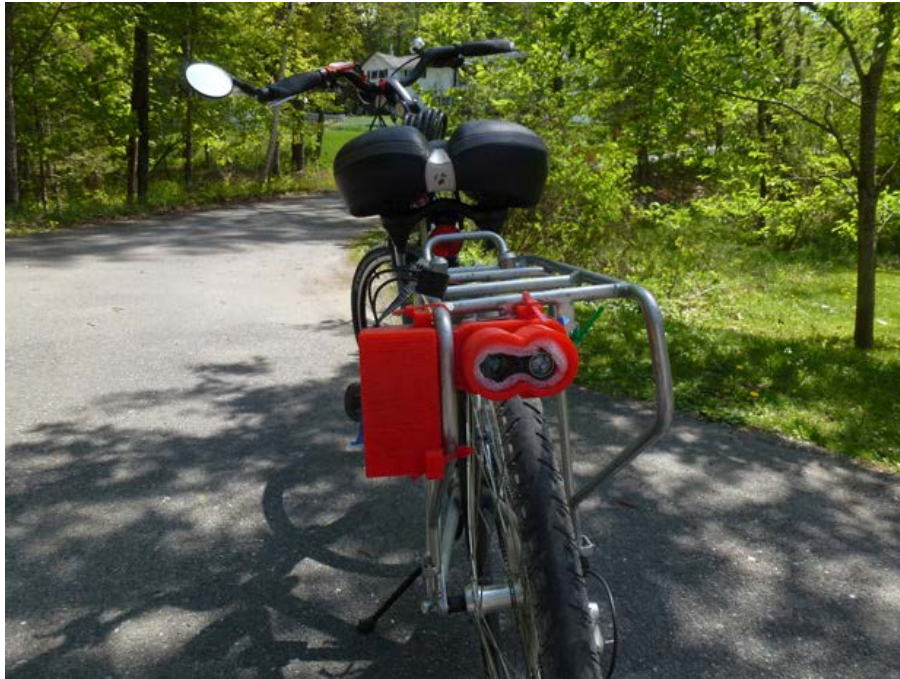
Figure 2.10 PulsedLight LIDAR-LITE v2 mounted on a bicycle.
