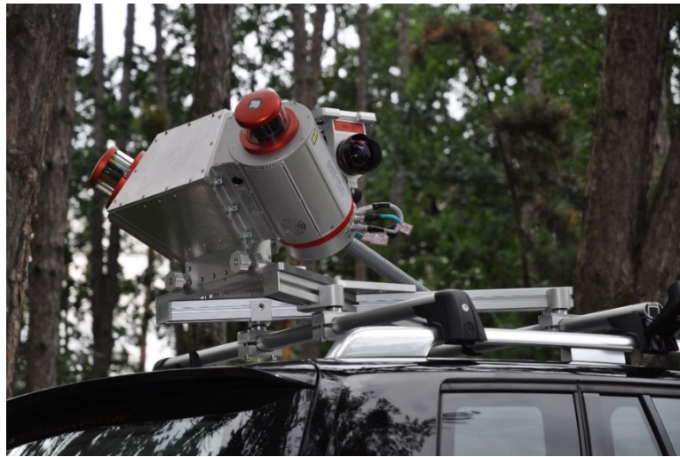
Figure 2.14 Riegl VMX-450 mounted on a vehicle.
