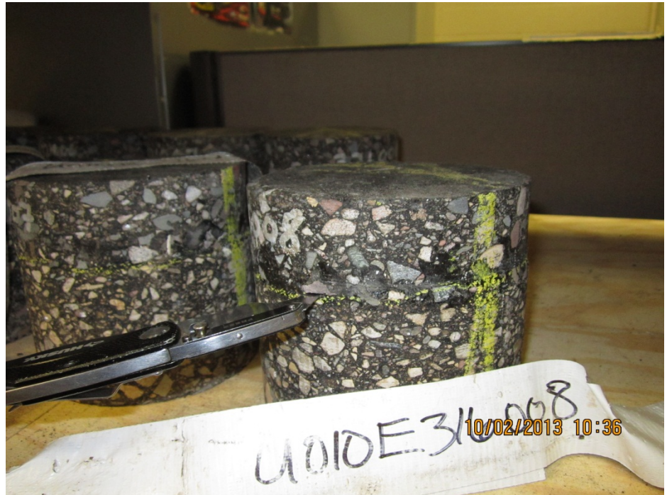
Figure - Typical Core after bond testing - Layers would require tools to separate. 0.24 g/sy PMAE pictured
