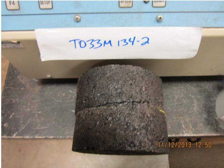
Figure - Gyratory mix specimens broken in shear device - notice apparent layer separation without a layer interface.
