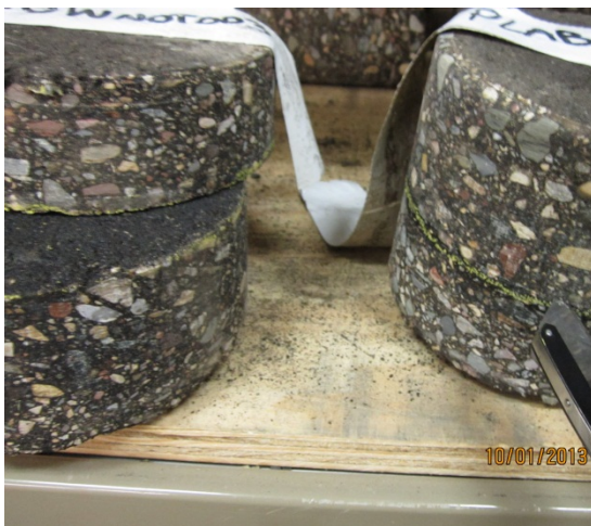
Figure - No-Tack Core (left) with clean layer separation. Tacked Core (right) was semi-bound after shear testing.
