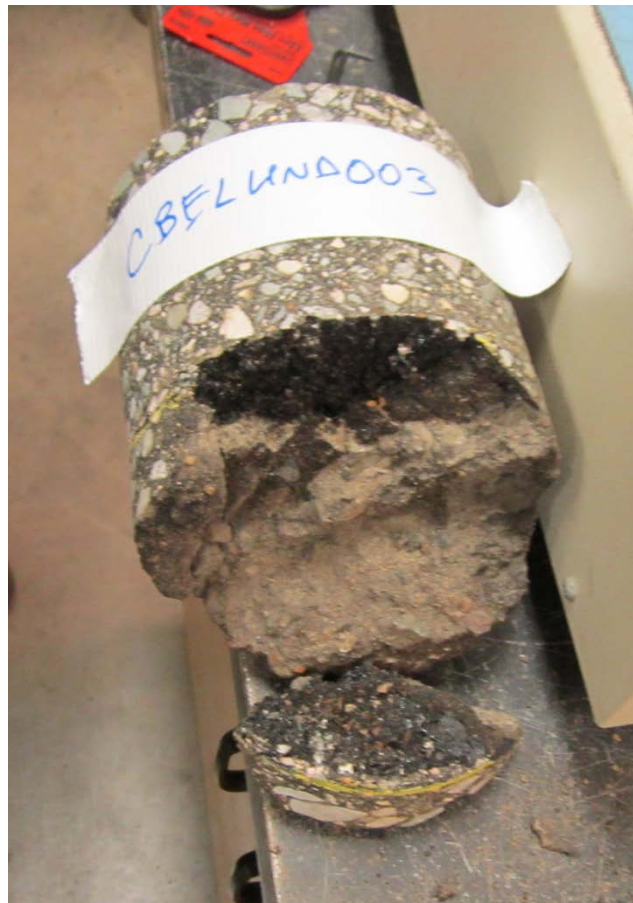
Figure - Underseal sample after testing.
