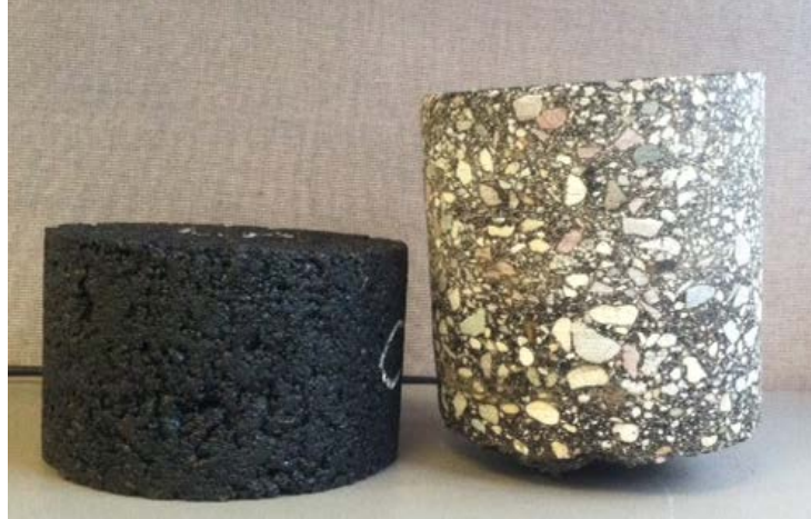
Figure 1.1: Gyratory pill (left) and field core (right).
