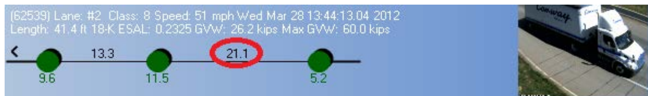
Figure 3.7. Correctly Classified Semi-Trailer Truck
