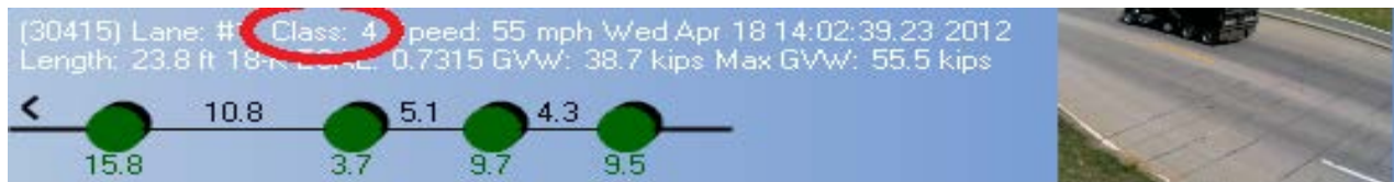
Figure 3.9. Class 7 Truck Misclassified as Class 4
