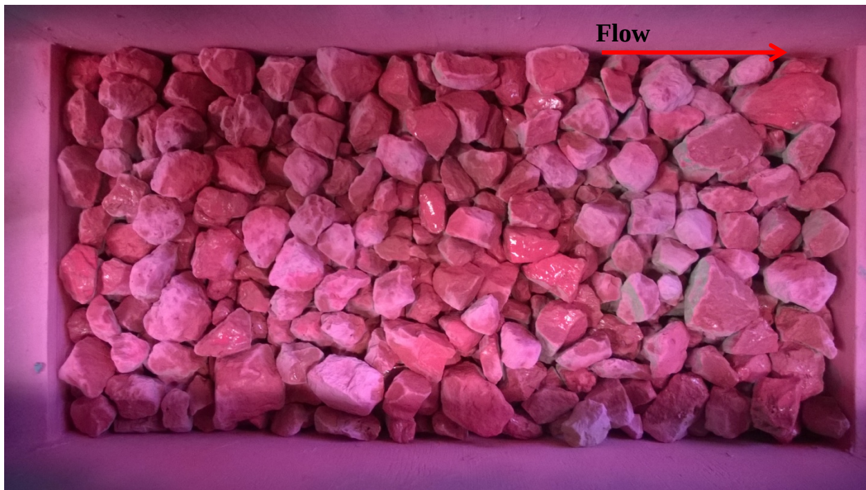
Figure 6.8. Pre-Run 1, 2-inch angular gravel with no grout.
