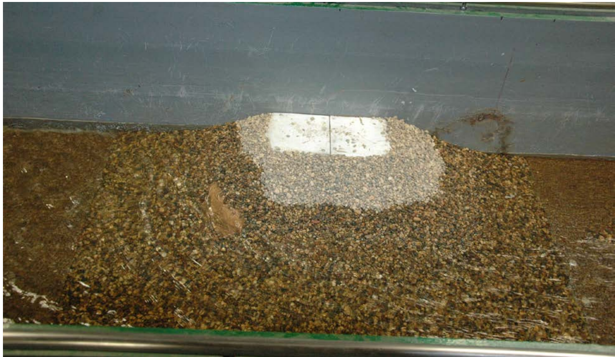
Figure 5.12. Flume setup for Model 1 with pea gravel.
