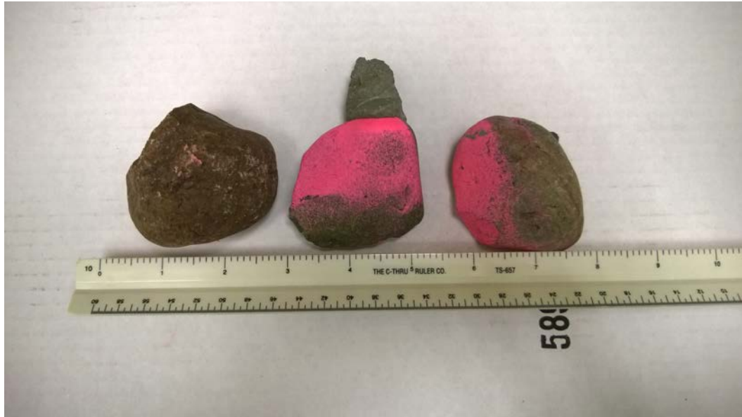
Figure 6.3. 2-inch river rock.
