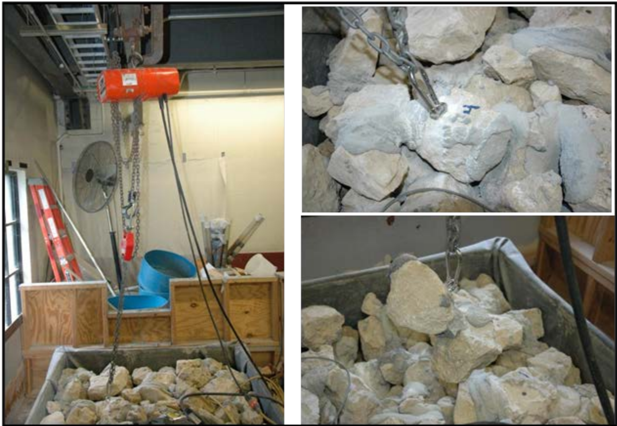
Figure 4.13. Mechanical pull test apparatus and anchoring system.
