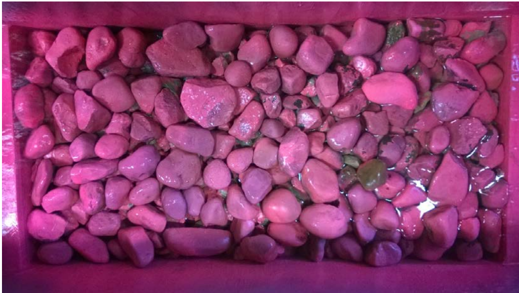
Figure 6.19. Post-Run 6, 2-inch river rock with no grout.
