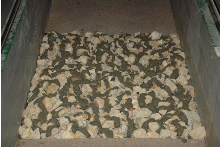
Figure 5.20. Plane bed configuration, matrix riprap.
