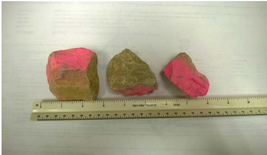
Figure 6.2. 2-inch angular gravel.
