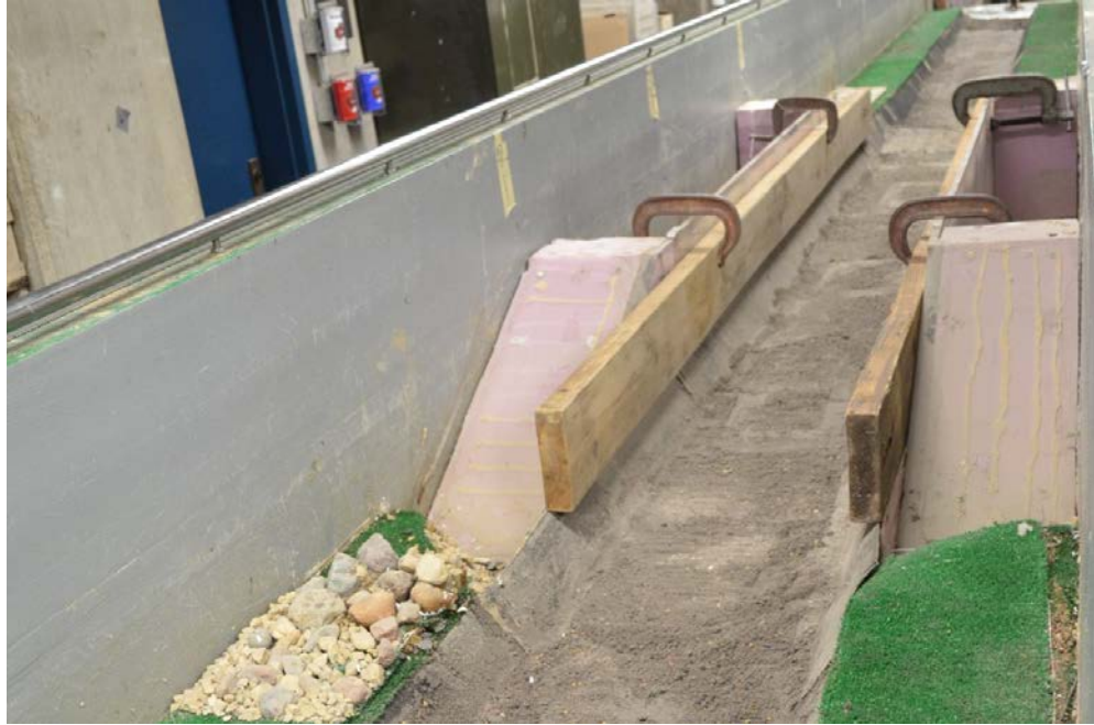
Figure 2.3. Pre-run equilibrium stream channel with temporary stream banks through culvert section. This image is from the fine sediment/low gradient experiments.
