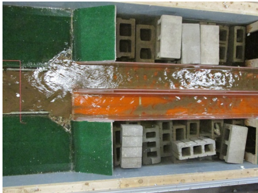
Photo 7: Bank Full Flow on Falling Limb
