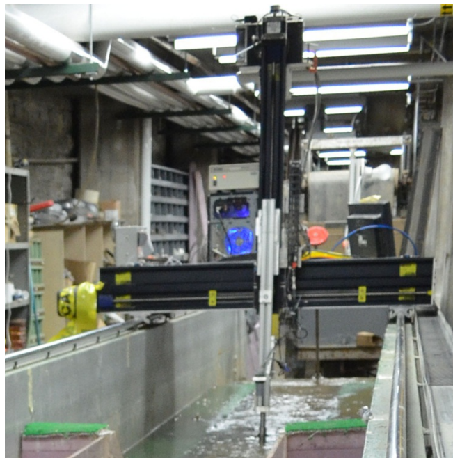
Figure 2.1. Instrumentation cart on the tilting bed flume with sonar, ultrasonic transducer, and laser range finder. This cart is also used to collect velocity measurements with an acoustic Doppler velocimeter (ADV).
