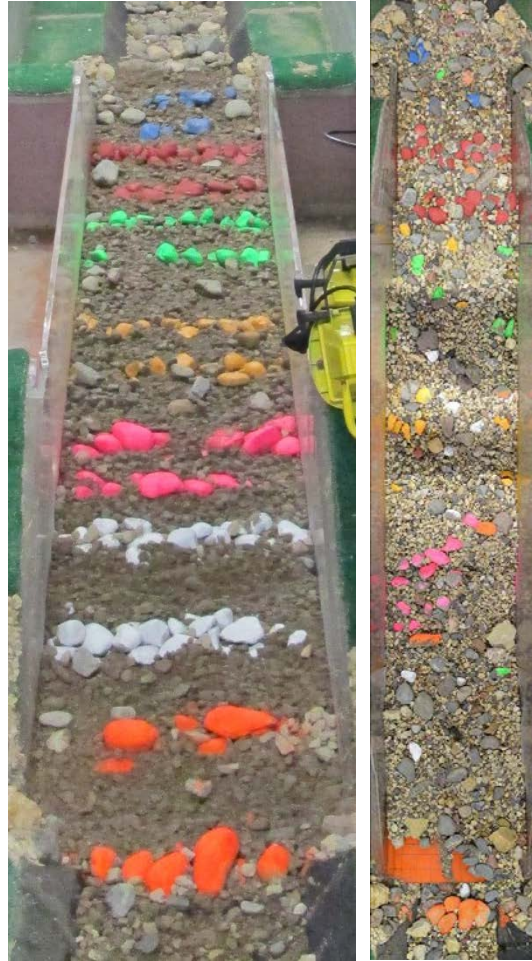
Figure 3.18. Pre- and post- photographs of structures placed in the culvert. Flow is from bottom to top. Each set of two structures was color coded to track the movement of structures.
