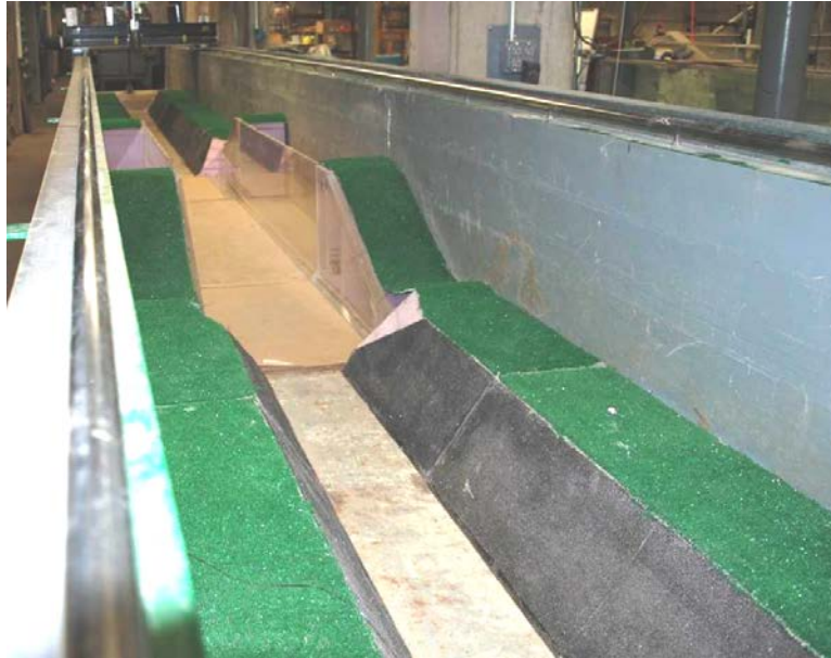
Figure 2.2. Model culvert and channel configuration in the tilting flume.
