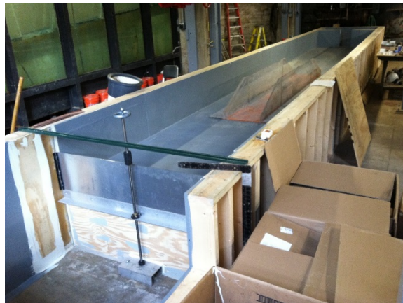
Figure 4.1. Image of multi-barrel testing facility and tailgate control design.
