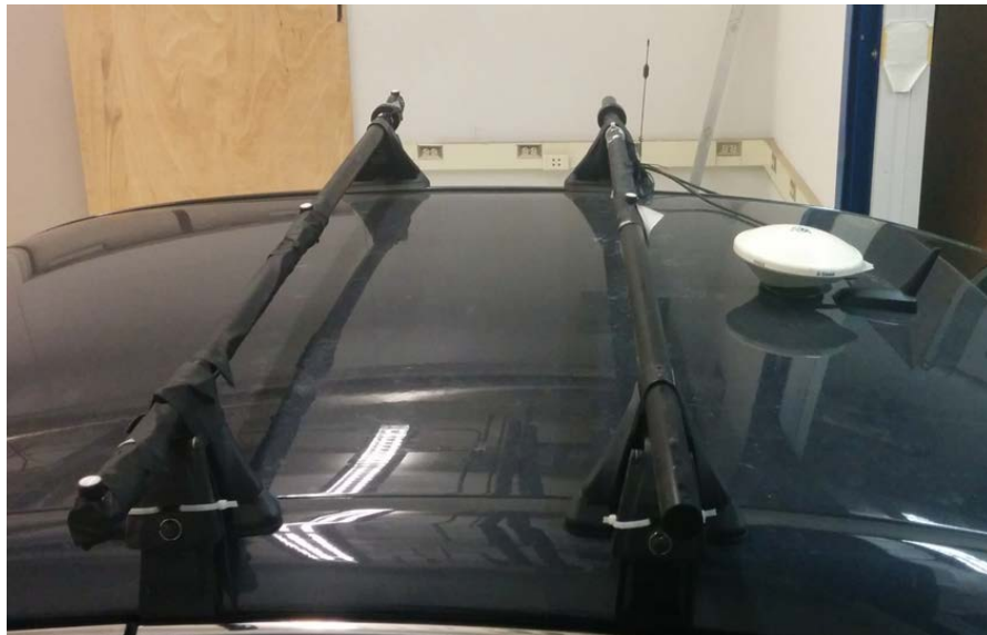
Figure 3. Illuminance measurement system with four visible heads (one positioned on the trunk) and the Trimble R7 GPS unit (white).
