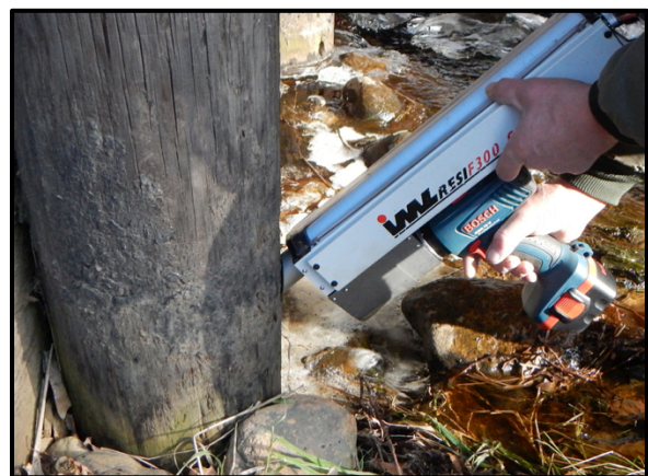
Figure 6.4. Drilling can take place at an angle to assess the area below ground line.
