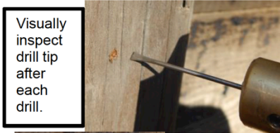
Silicone should be used to fill the tiny hole.
