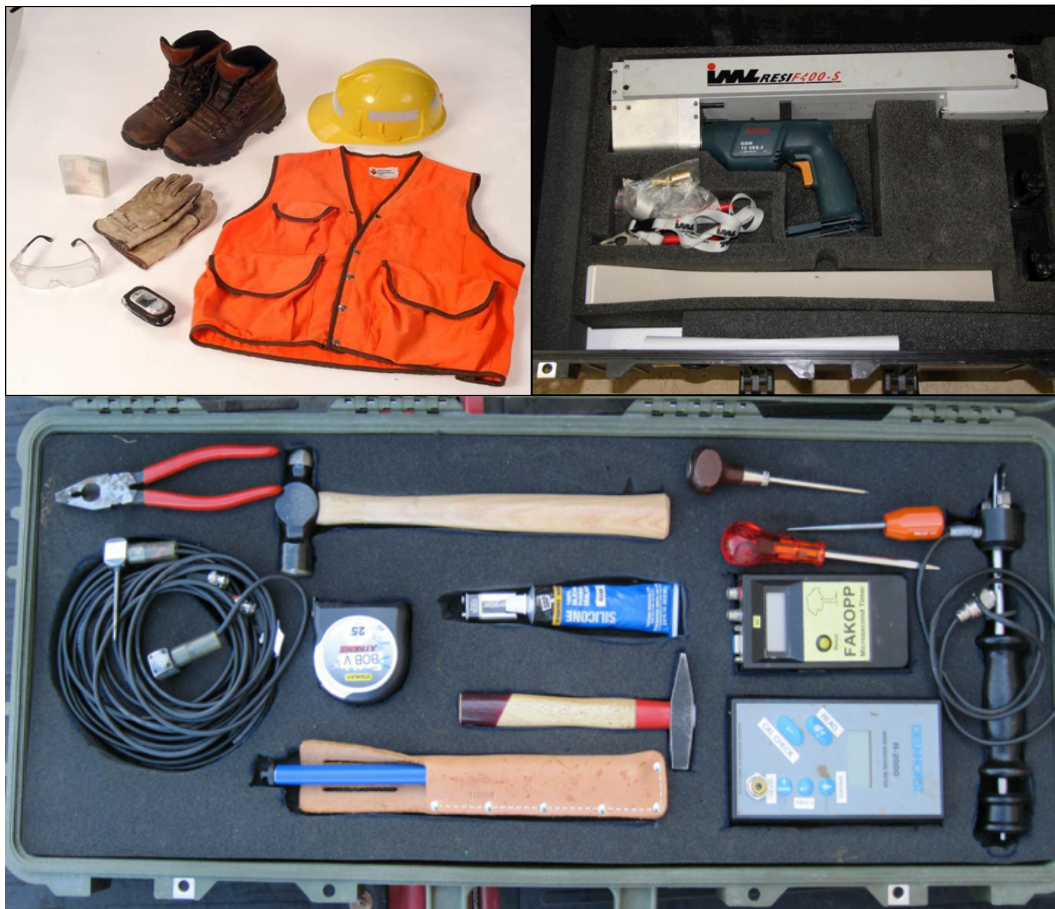
Figure 2.1. Inspection equipment used for inspecting timber bridges.
