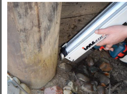
A 45° attachment allows for inspection below the water or ground line. Silicone should be used to fill the hole.
