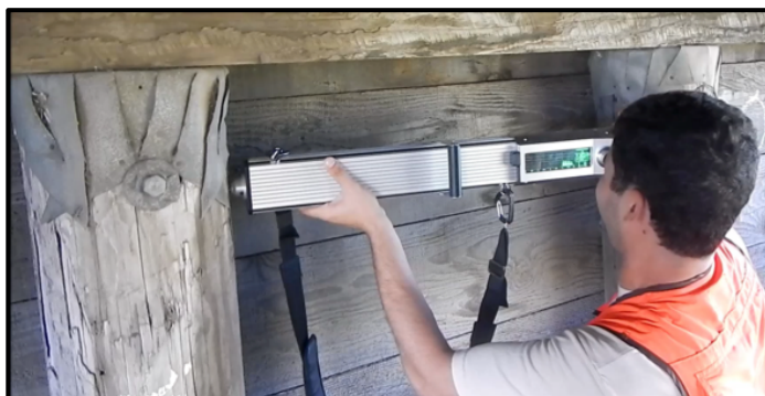
Figure 6.6. Electronic display on a resistance drill.
