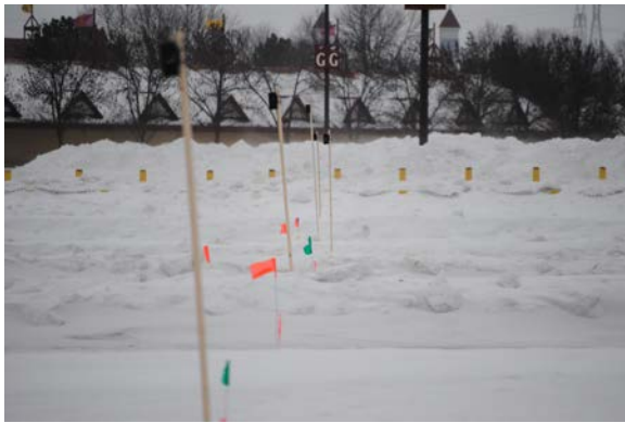
c) Pole mounted cameras directly inserted into plow windrows.
