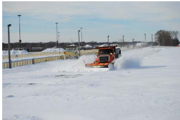
d) CD4 at 20 mph, front plow angled left.
