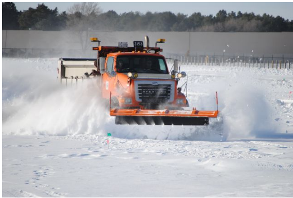
a) MnDOT tandem axle dump truck with front and right wing plows engaged.
