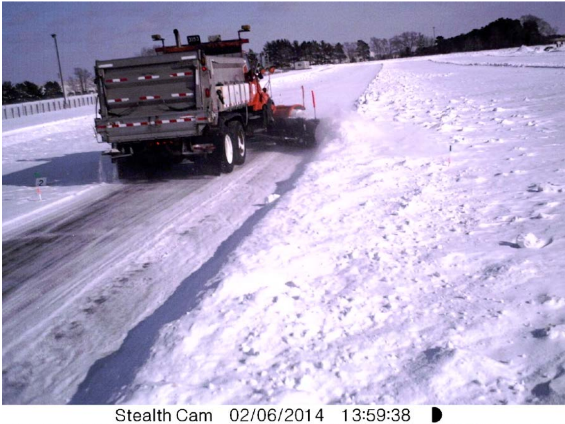
Figure 34. Typical time lapse photograph showing front and wing plowing plus deicer application (left rear distributor). Notice difference of scrape quality between front plow (directly behind truck) and wing plow. Prior to December 18, 2013, snow remaining the day after a storm event was insufficient for testing and evaluation. On March 6, 2014, an additional day of plowing and deicing was planned; however, melting of snow created slick conditions underlying the snow. A MnDOT truck mounted plow was unable to clear access to the pavement lanes at Canterbury Park, resulting in test cancelation. By March 13, 2014, insufficient snow remained on the pavement lanes for additional testing.
