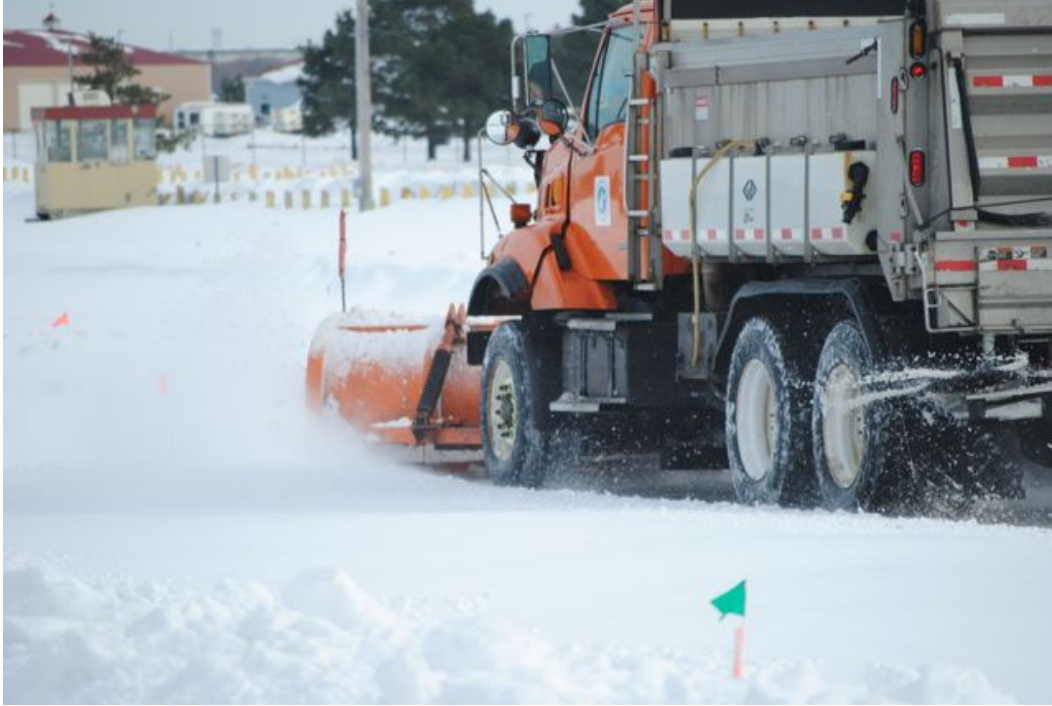
Figure 23. MndOT truck spreading deicer off left rear while moving forward with a right-angled front plow.
