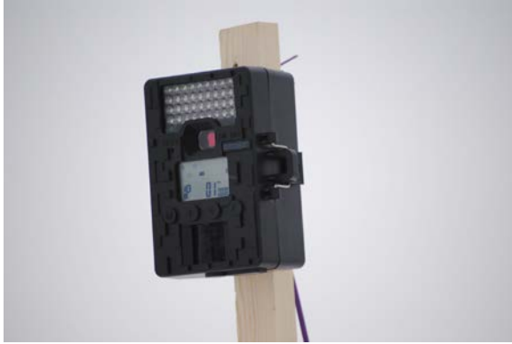
a) Time-lapse camera, pole mounted.
