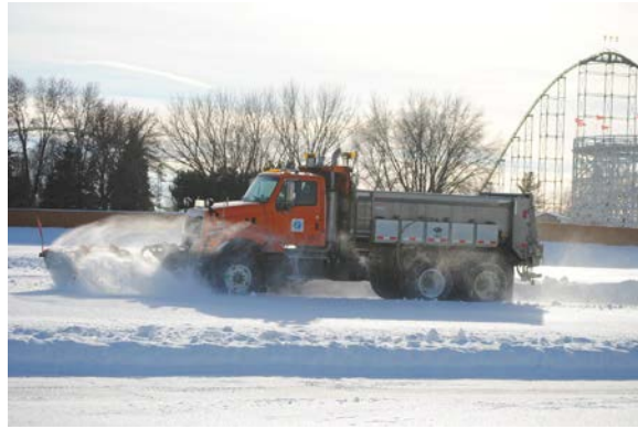
b) MnDOT truck with saddle tanks for prewet fluid.
