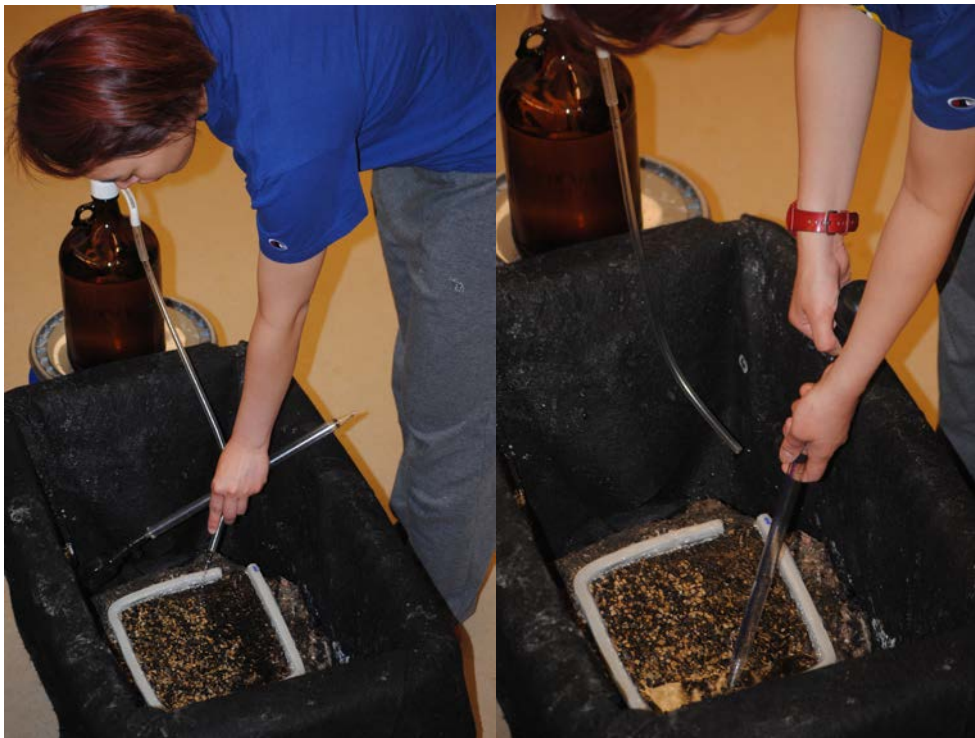
Figure 45. Precipitation water application (left) and drainage collection (right).
