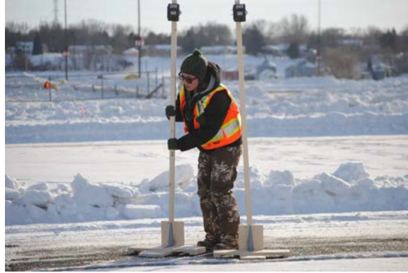
b) Pole mounted cameras with detachable bases being deployed.
