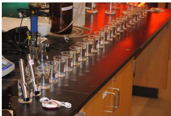
b) Calibration mixtures lined up for measurement by data loggers.
