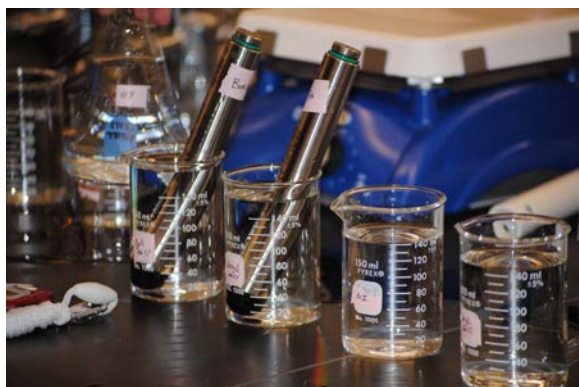
a) Two data loggers in calibration mixtures.
