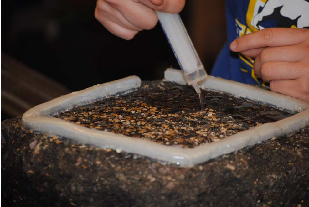
Figure 44. Anti icer application to defined pavement area.
