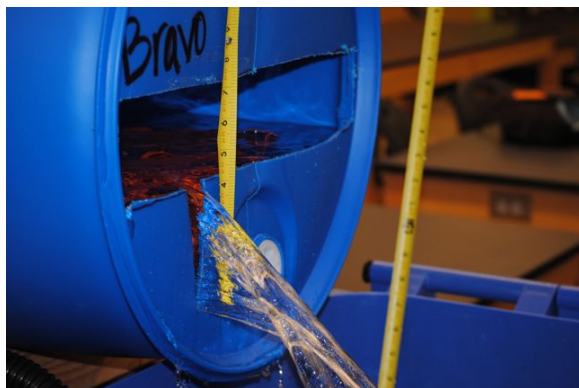
a) Flow-through V-notch weir into receiving sump.
