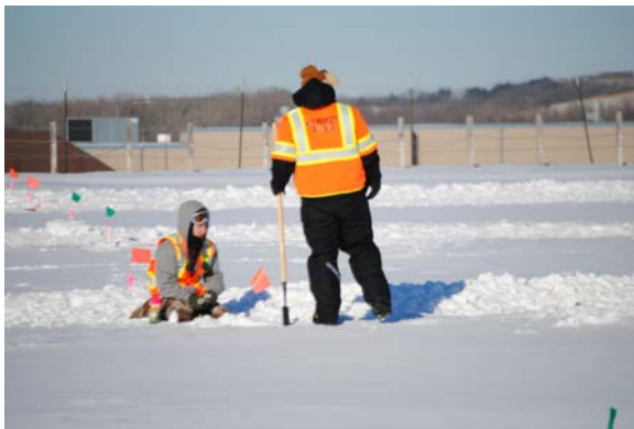
Figure 27. Placement of lane marking flags and stationing of lane distance.
