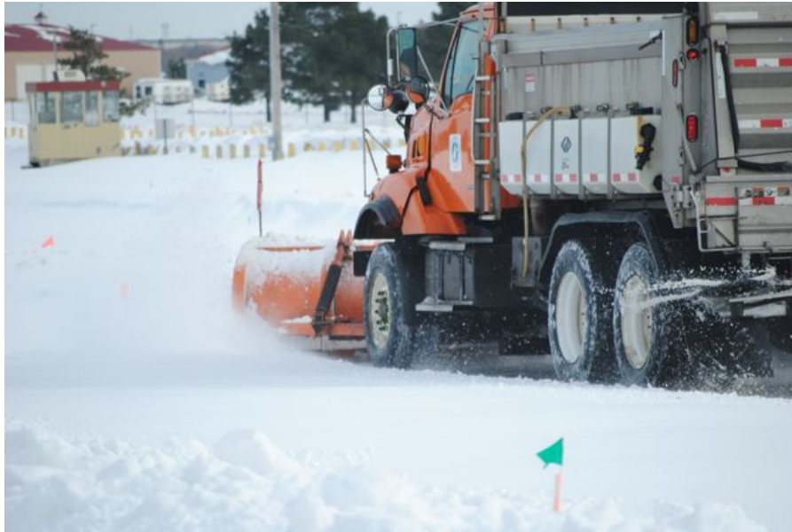
a) MnDOT truck spreading solid deicer with prewet off left rear.
