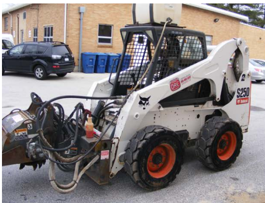
(a) Miller attached to Bobcat loader
