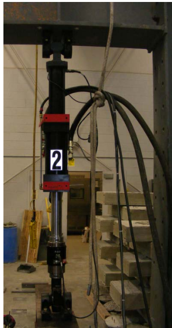
Figure 3-20 35-kip capacity hydraulic actuator, fully extended
