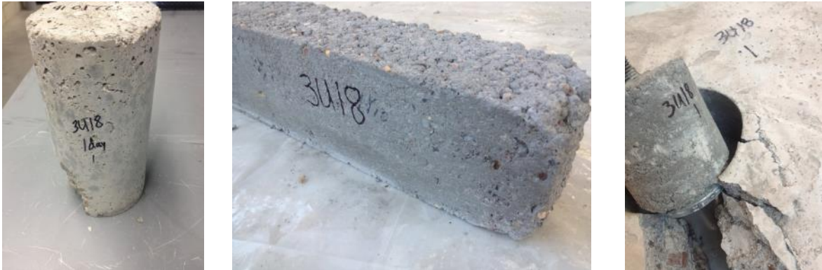
Figure 35: 3U18 compression, freeze thaw and pull out specimens
