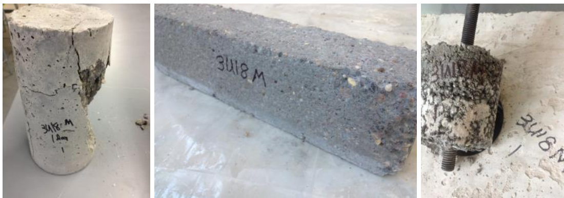
Figure 36: 3U18M compressive, freeze-thaw and pull out specimens
