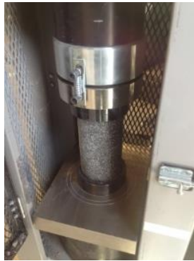
Figure 2: Compression Test Setup
