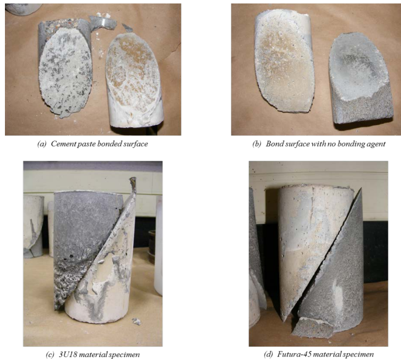
Figure 4-1 Photographs of slant shear specimens after failure
