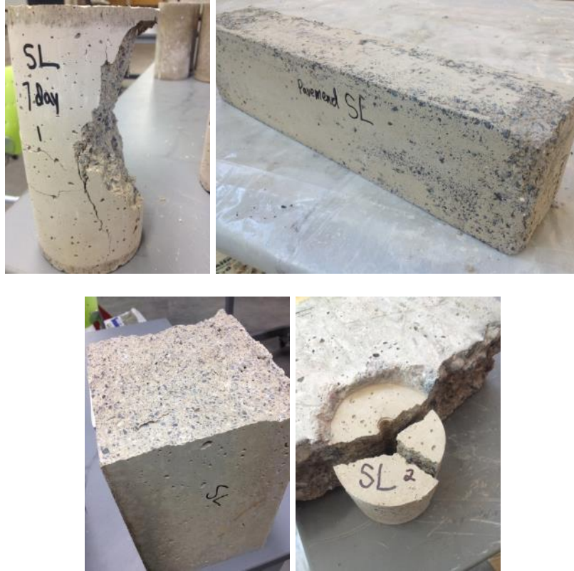
Figure 44: Pavemend SL compressive, freeze-thaw, flexural and pull out specimens
