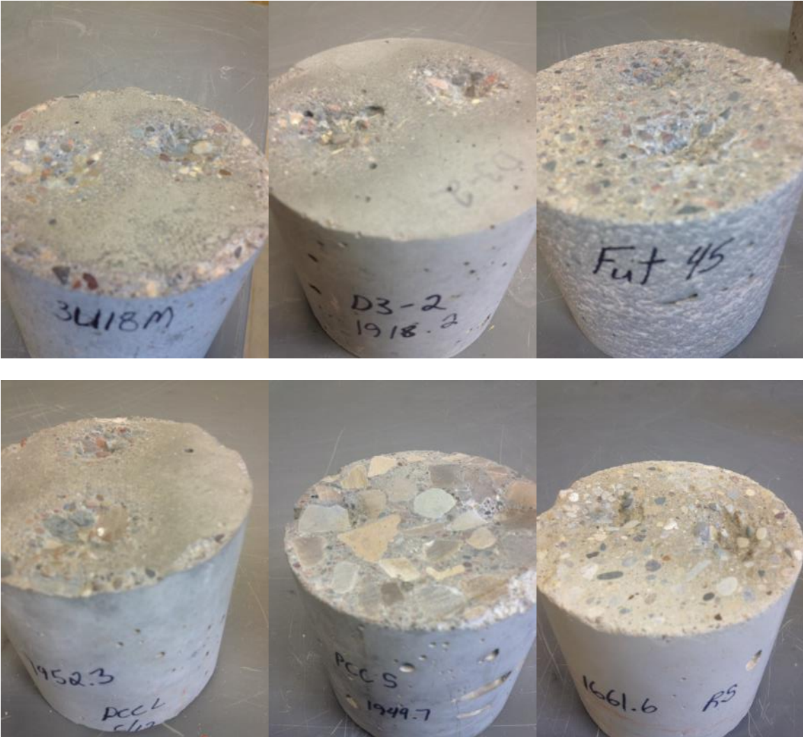
Figure 56: Abrasion test specimens.
