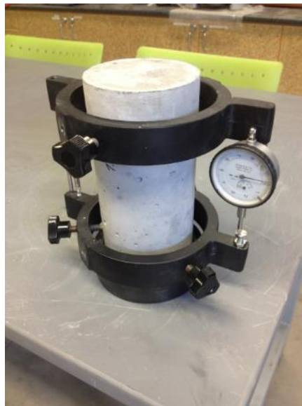
Figure 9: Modulus of elasticity apparatus with dial gage.
