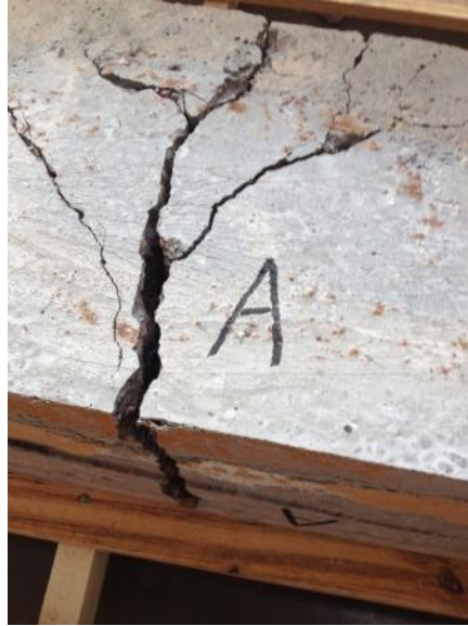
Figure 64: Specimen “A” (D3-2-W) exhibiting central crack propagation.
