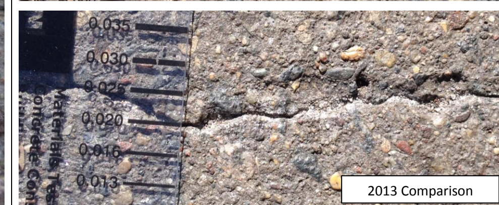
Photograph #: 6 Test Information: Test Section 1, Test 2A - Accuflex Coatings Gel-Seal (Silicate) Surface Prep & Application: Air Hose, Pretreat, Flood, Sand Coat: No Date: April 8, 2014 BRAUN INTERTEC
