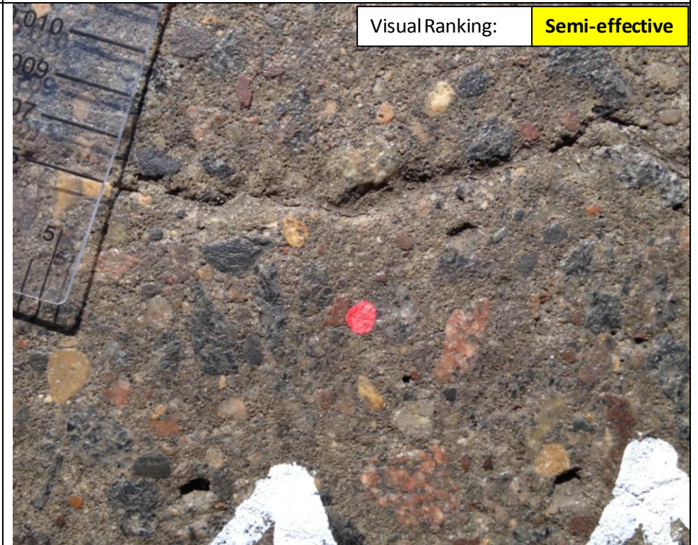
Photograph #: 24 Test Information: Test Section 4, Test 10B - TK Products TK-2110 (Epoxy) Surface Prep & Application: Sand Blast, Flood, Sand Coat: Yes Date: April 8, 2014 Project BL-09-03973 BRAUN INTERTEC
