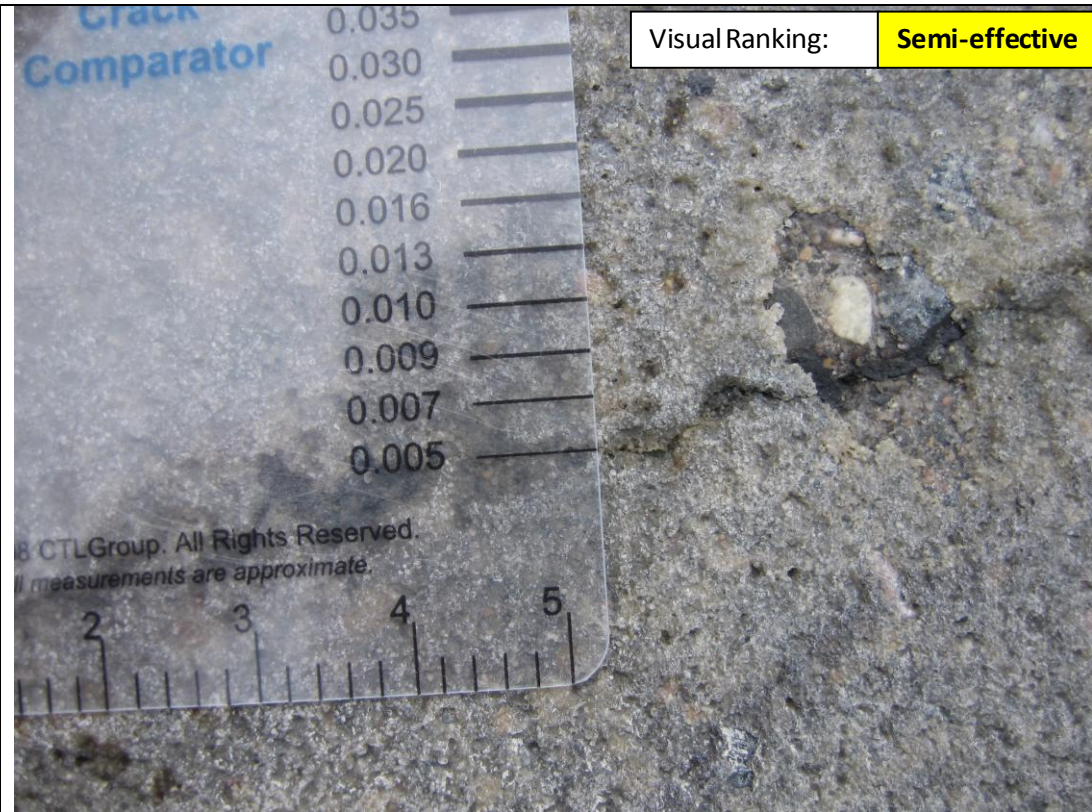
Photograph #: 20 Test Information: Test Section 4, Test 9A - TK Products TK-2110 (Epoxy) Surface Prep & Application: Air Hose, Flood, Sand Coat: Yes Date: April 30, 2013 Project BL-09-03973 BRAUN INTERTEC
