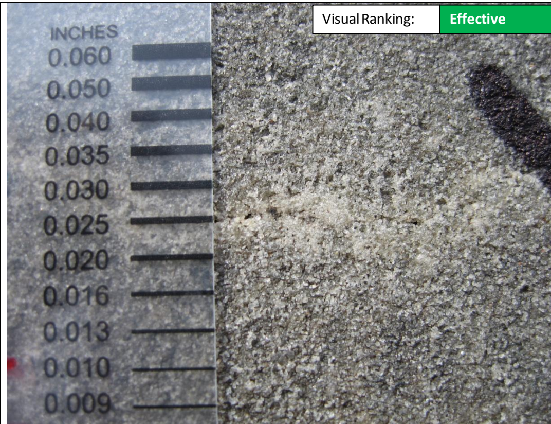
Photograph #: 73 Test Information: Test Section 13, Test 25A - Euclid Chemical Dural LM 50 (Epoxy) Surface Prep & Application: Air Hose, Pretreat, Bottle (squeegee), Sand: Yes Date: May 11, 2012 Project BL-09-03973 BRAUN INTERTEC
