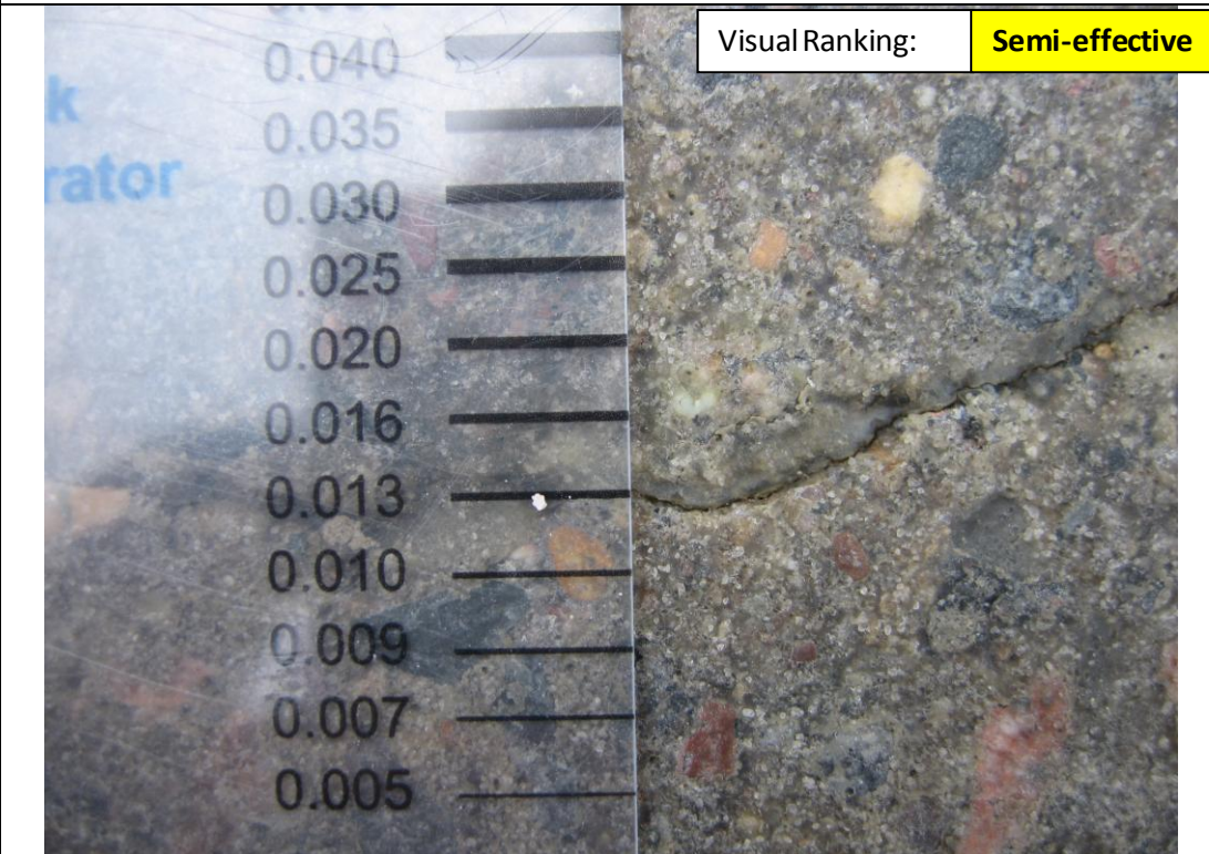
Photograph #: 23 Test Information: Test Section 4, Test 10B - TK Products TK-2110 (Epoxy) Surface Prep & Application: Sand Blast, Flood, Sand Coat: Yes Date: April 30, 2013 Project BL-09-03973 BRAUN INTERTEC
