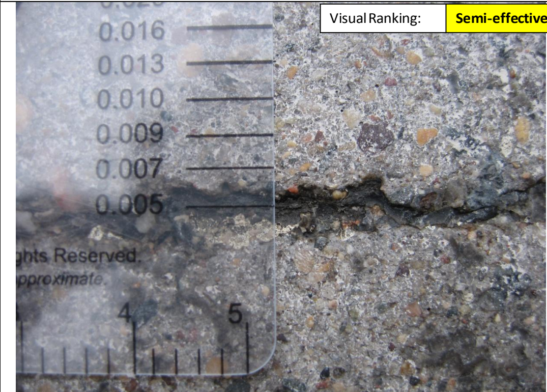
Photograph #: 47 Test Information: Test Section 8, Test 20A - Kwik Bond KBP 204 P (HMWM) Surface Prep & Application: Air Hose, Flood, Sand Coat: Yes Date: April 30, 2013 Project BL-09-03973 BRAUN INTERTEC
