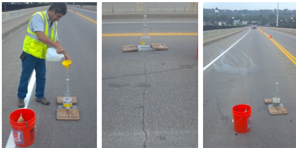
Figure 6. Crack Permeability Testing on the Smith Avenue High Bridge
