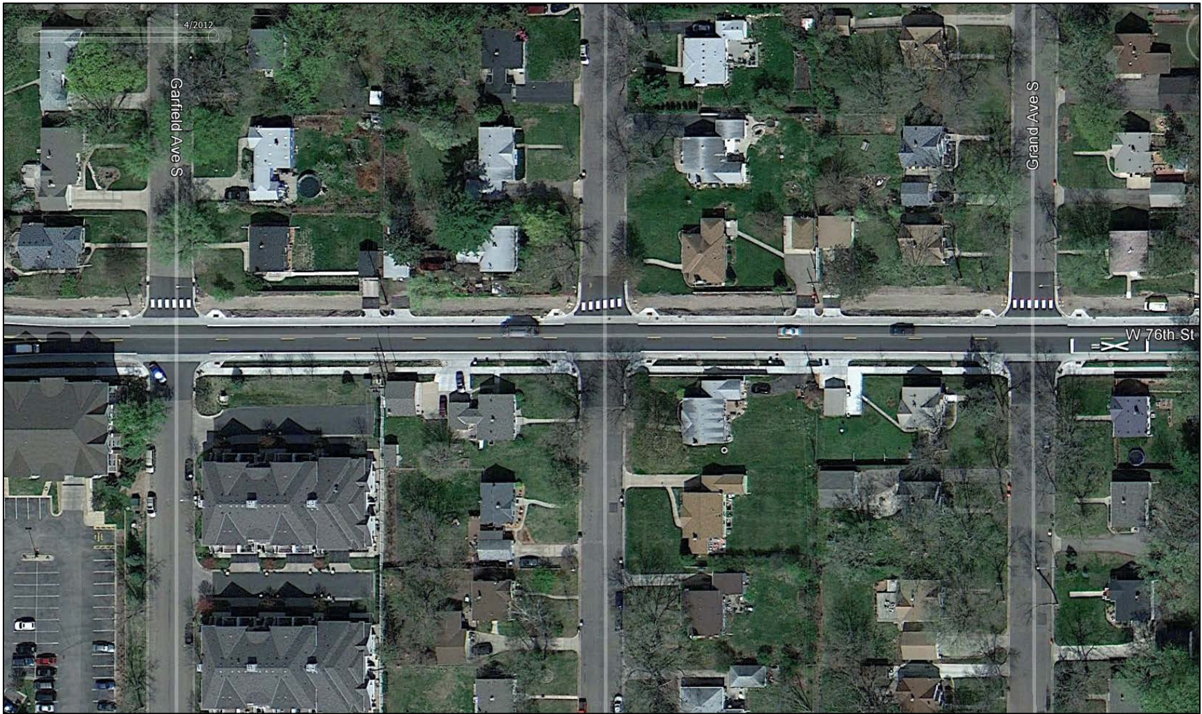
Figure 4.19: Example of 76 th Street Section (Between Garfield and Grand Avenues) After Reconstruction Showing Two-Lane Roadway with In-Road Bicycle Lanes and Multi-Use Path
