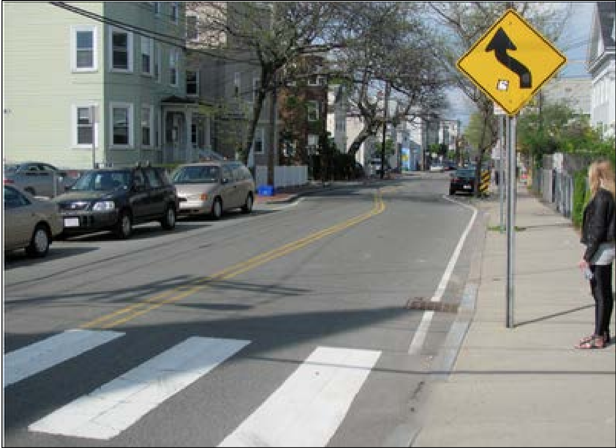
Figure 2.10: Alternate On-Street Parking Creates Chicane [18]
