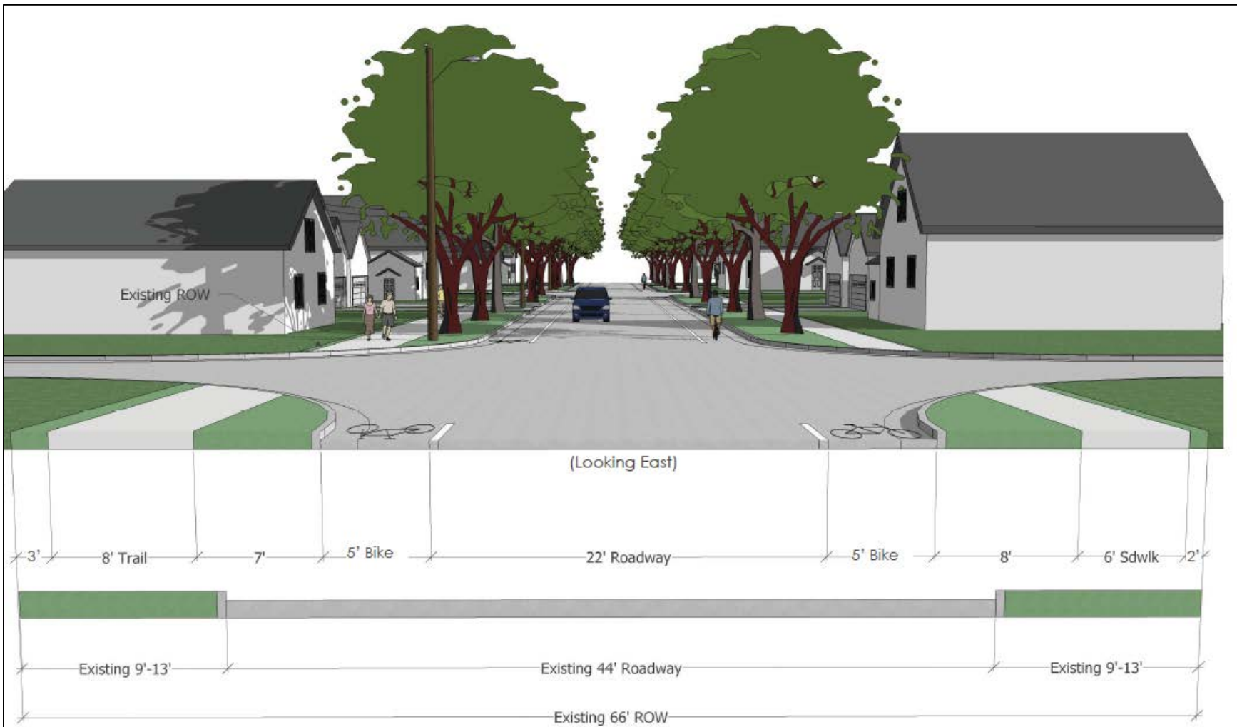
Figure 4.17: Right-of-Way Allocation for 76 th Street between Xerxes and Lyndale Avenues Before and After Reconstruction Source: City of Richfield, Minnesota, Howard R. Green Company.
