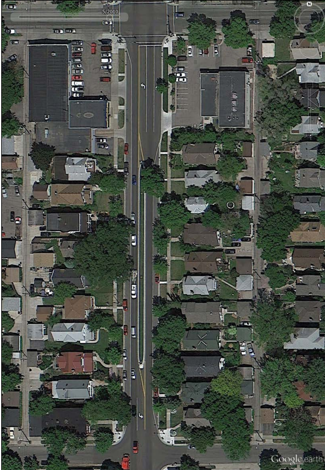
Figure 4.6: Example of Lyndale Avenue (36 th and 37 th Street Block) After Reconstruction Showing Raised Median, Delineated Parking Lanes, and Exclusive Left-Turn Lanes
