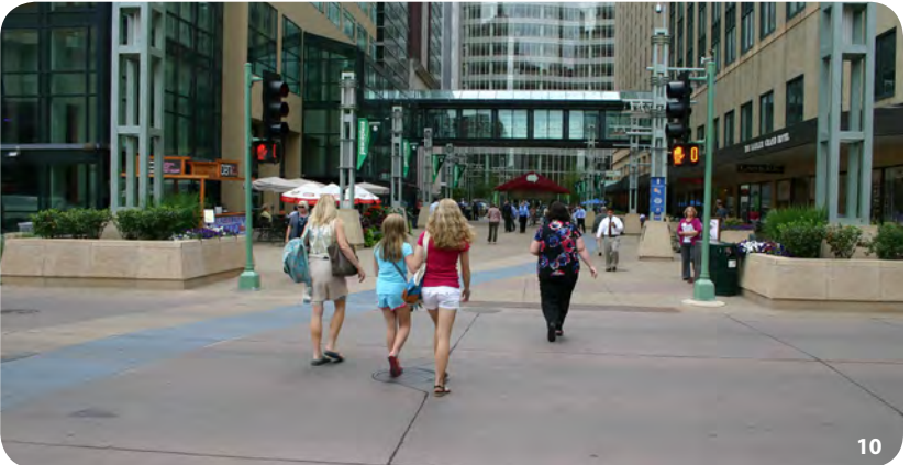
10. As the plaza intersects with 1st Avenue the pedestrian crossing is at grade, meaning pedestrians do not have to surmount a curb or ramp to cross the street. It is a wide crosswalk with colored concrete and timed crossing lights.
