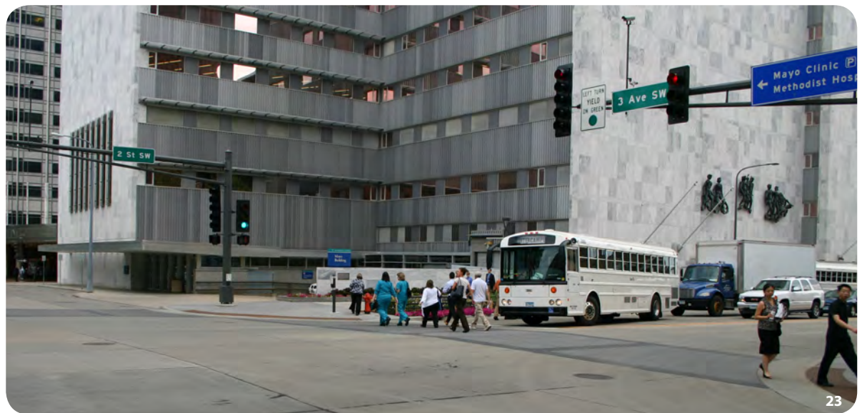
23. Wide curb cuts and wide crosswalks along 2nd Street and 3rd Avenue provide good accessibility for wheelchairs and allow for larger groups of pedestrians to cross together.
