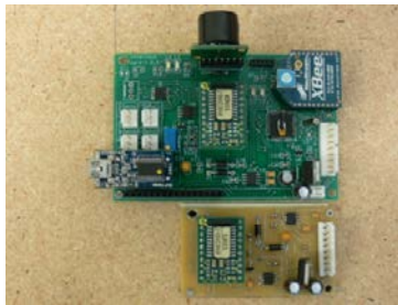
Figure 2.1: PCB with two AMR sensors, microprocessor and wireless transceiver system
