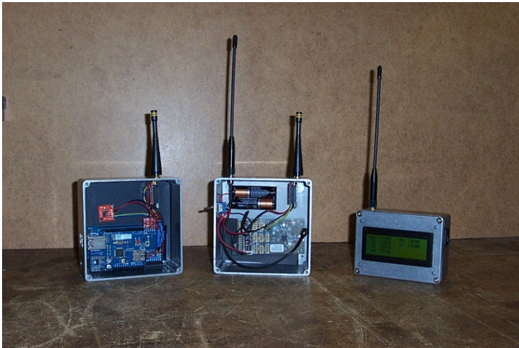
Figure 4.4: Showing internals of interface components for WIM sensor
