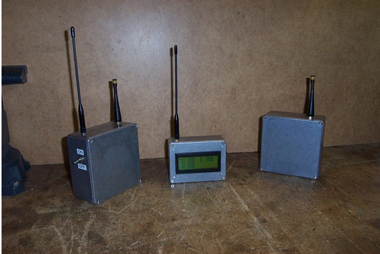
Figure 4.3: Major interface components for access to WIM sensor
