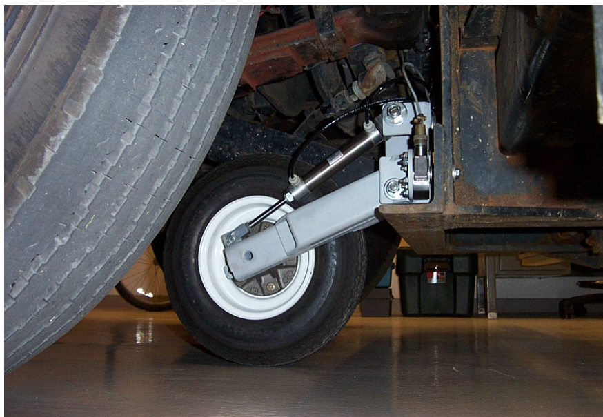
Figure 1: Friction measurement wheel installed on a snowplow.
